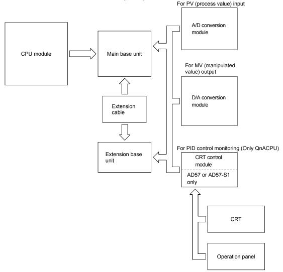
SV, PV and MV used with the PID control instructions may be set either with the fixed values of 0 to 2000 or to any values according to the used module. Refer to Section 4.3.5 for details.
