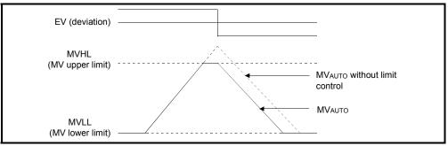
Fig. 4.6 Operation in Accordance with the MV Upper/Lower limit
