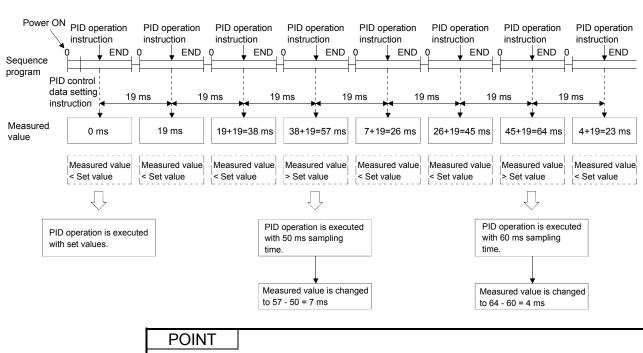
The sampling cycle is measured when the PID operation instruction is executed. Therefore, a value smaller than the sequence program scan time cannot be set for the sampling cycle. If a value smaller than the scan time is set, PID operation will be executed in accordance with the scan time.
