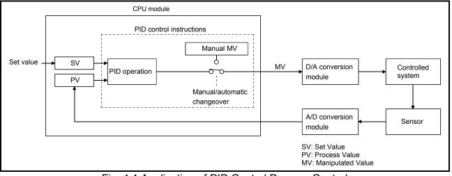
Fig. 4.1 Application of PID Control Process Control
