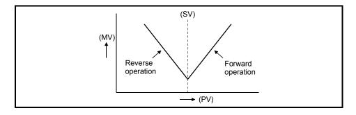
(5) The figure below shows examples of process control with forward operation and reverse operation:
