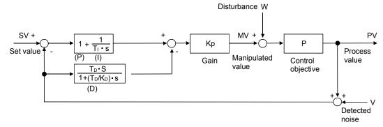
(1) The PID operation block diagram for incomplete derivative is shown below.
