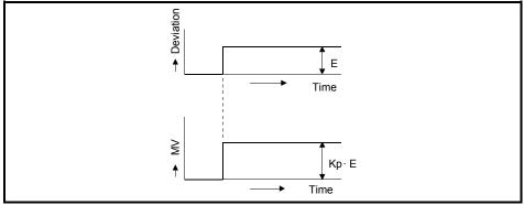
Fig. 4.2 Proportional Operation with a Constant Deviation
