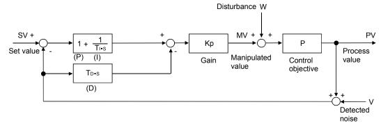
(1) The PID operation block diagram for complete derivative is shown below.
