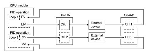
Q64AD I/O numbers ......X/Y80 to X/Y8F Q62DA I/O numbers .....X/YA0 to X/YAF
