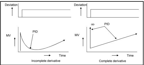
Fig. 4.5 PID Operation with Constant Deviation
