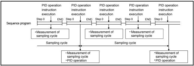
Figure 1. 2 Operation when PID Operation Instruction Executed
