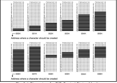
Fig. 9.1 Characters for PID Control Status Monitor
