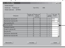
This single line is counted as one parameter that has been set. A blank is counted out.
