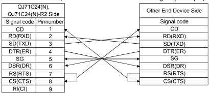
Connection example which cannot turn ON/OFF CD signal (No. 1 pin)
