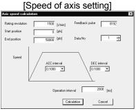
These functions allow the optimum positioning data to be set without complicated calculation and advance measurement.
