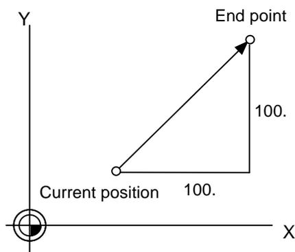
**(Example) Non-linear type** (Each axis moves with each parameter speed.)
