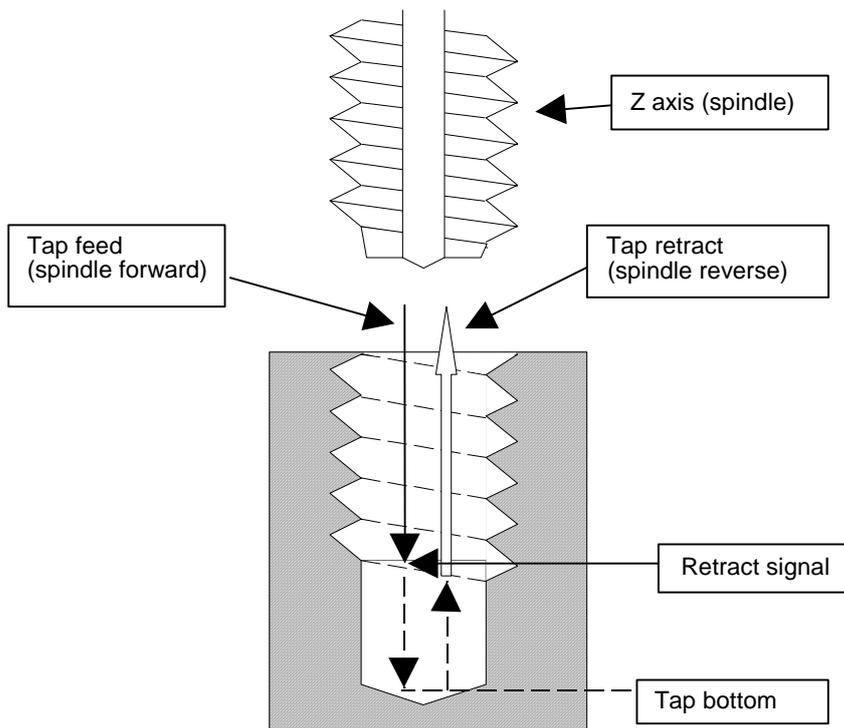
This function can be used by an interruption initiated by reset or emergency stop. A return is made to the initial point by tap retract.
