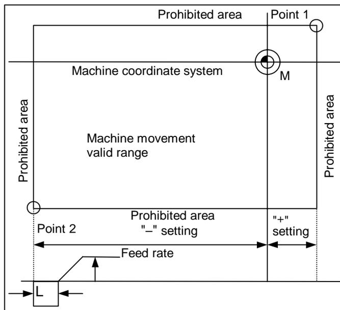
The values of points 1 and 2 are set using the coordinate values in the machine coordinate system.
