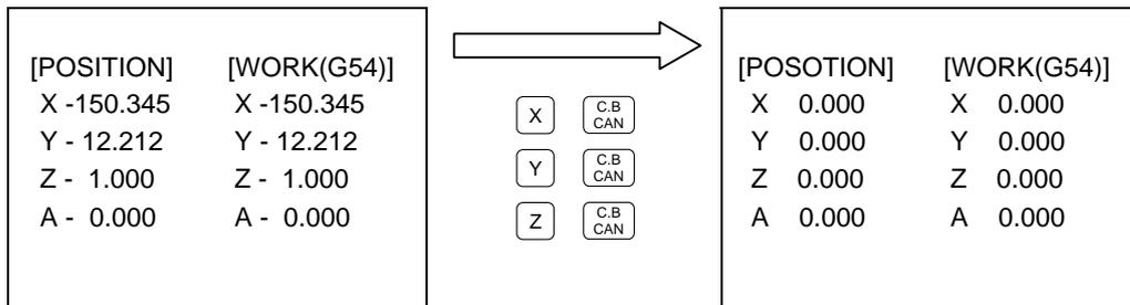
When axes are set to "0" in order, the Y and Z axis can be set by pressing key successively without pressing and keys.
