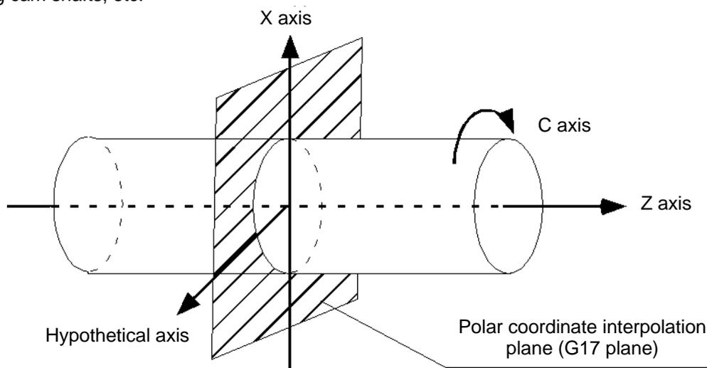
Fig. 1 Diagram explaining polar coordinate interpolation axes
