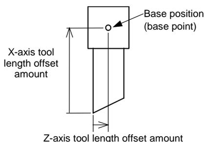
2. The programmed base position is the tip of the base tool:
