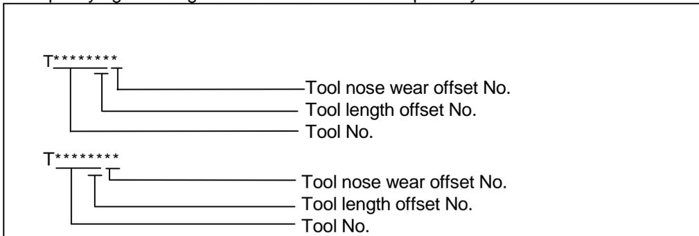
The tool offset for the lathe is valid only for the X and Z axes. If the 3rd axis (Y axis) is added, the tool offset will be validated for the 3rd axis.
