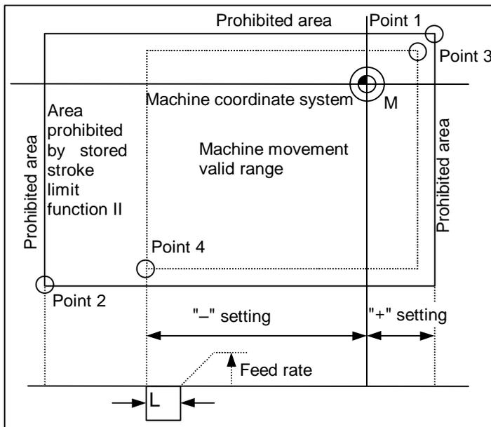
The values of points 3 and 4 are set with the coordinate values in the machine coordinate system.
