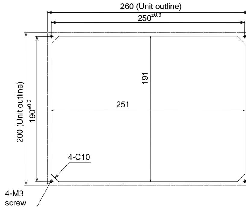
How to fix with screws from the front of the unit (Reference)
