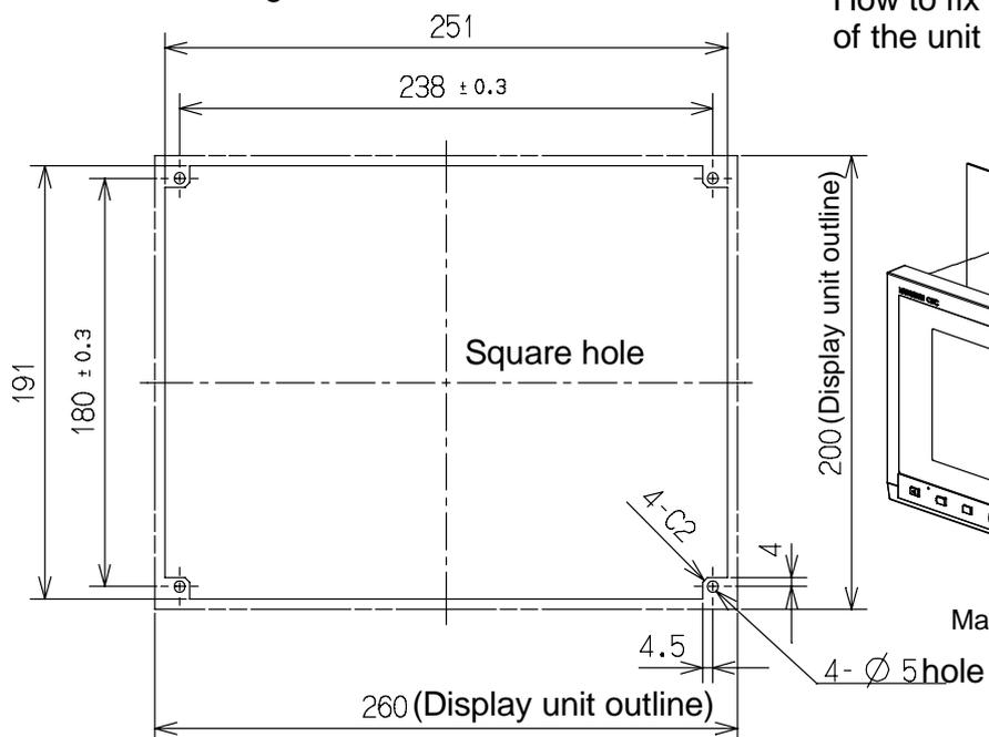
How to fix with screws from the back of the unit (Reference)
