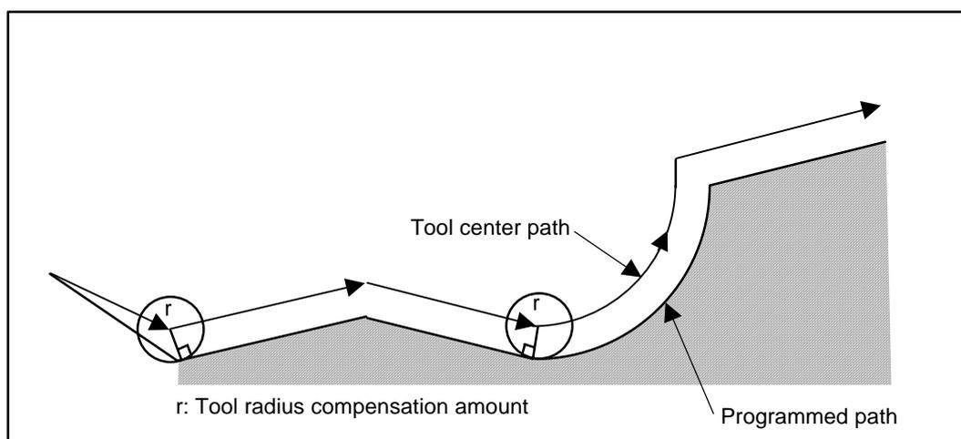
The tool radius compensation command controls the compensation from that block in which G41 or G42 is commanded. In the tool radius compensation mode, the program is read up to five blocks ahead including blocks with no movement, and interference check using tool radius is conducted up to three blocks ahead in any of those blocks with movement.
