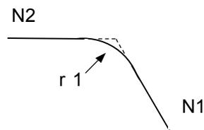
**(Note 1)** If a corner chamfering or corner rounding command is issued specifying a length longer than the N1 or N2 block, a program error occurs.
