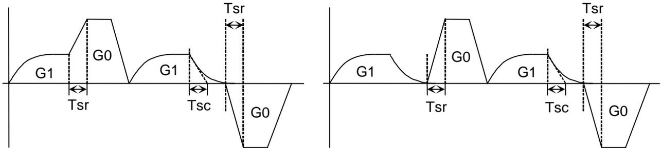
If the G0 command direction is the same as that for G1, whether G1 is to be decelerated is selected using a parameter.
