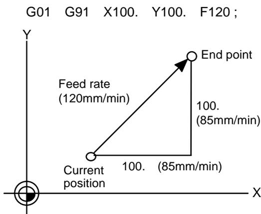
1. The cutting feed rate command moves the tool in the vector direction.
