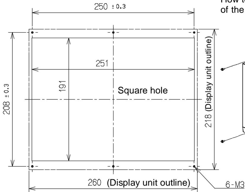
How to fix with screws from the front of the unit (Reference)
