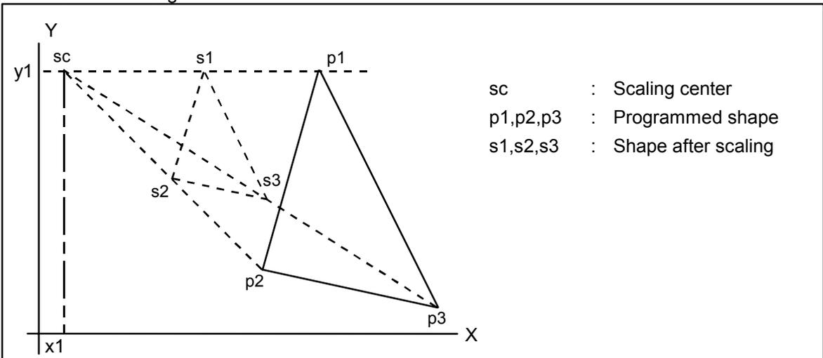
**(Note 1)** Scaling cannot be applied to compensation amount for tool radius compensation, tool position offset, or tool length compensation, etc. (The compensation and offset are calculated for the scaled shape.)
