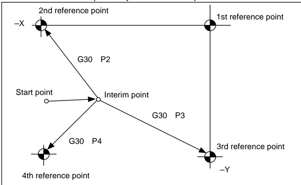
**(Note 1)** The second reference position return is performed if the P command is omitted.
