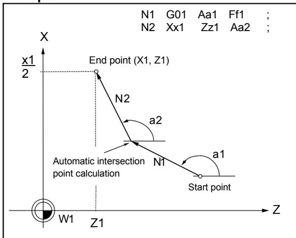
a: Angle (°) formed between straight line and horizontal axis on plane.
