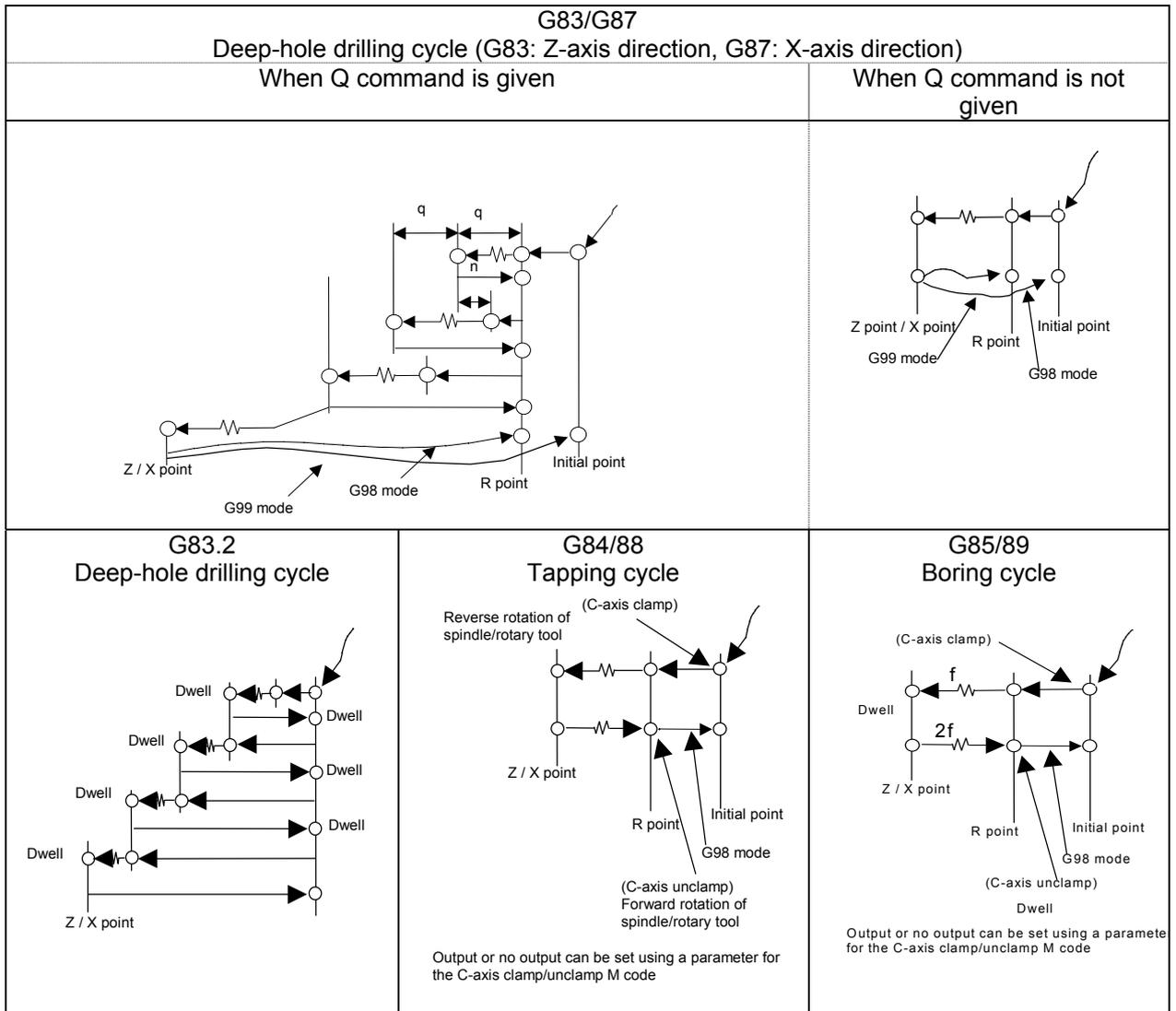
There are two levels of hole machining axis return which apply upon completion of the fixed cycle machining operation. (see the figure above)
