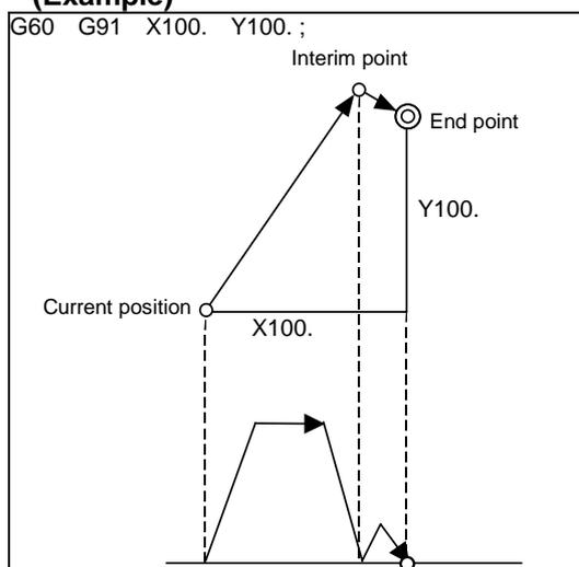
1. The rapid traverse rate for each axis is the value set with parameters as the G00 speed.
