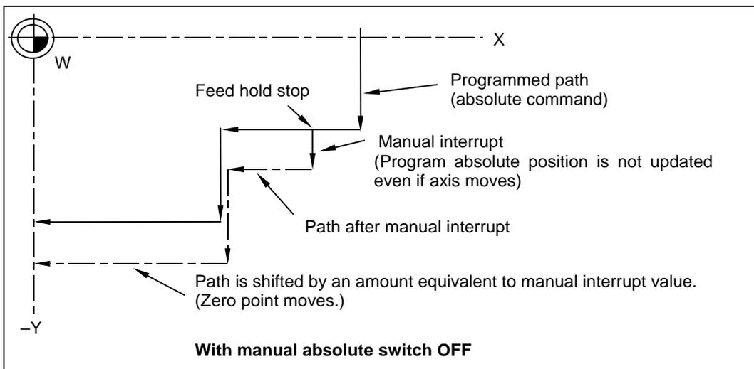
The switch ON state will be entered when the power is turned ON.
