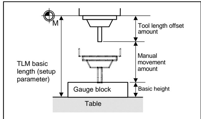
If the height axis designation parameter is ON, the axis designated for plane selection basic axis K is the axis targeted for measurement as the height axis.
