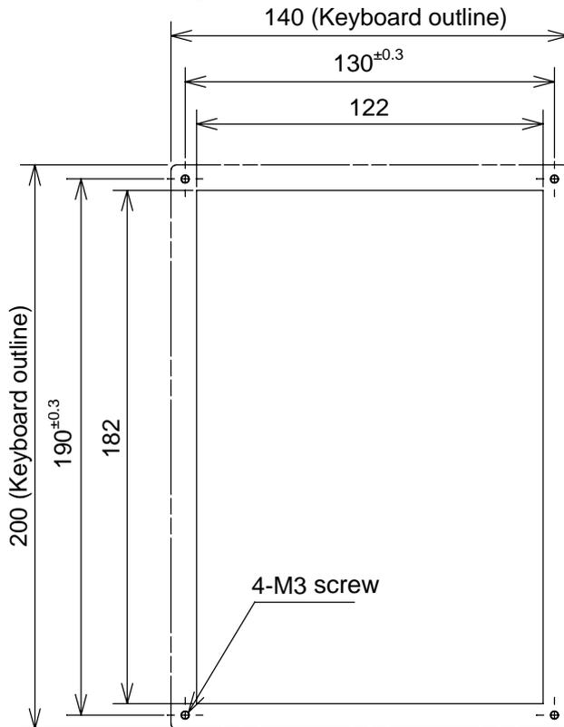
How to fix with screws from the front of the unit (Reference)
