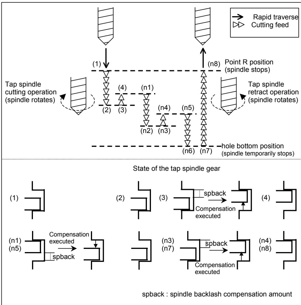
(Note) In the deep-hole tapping cycle, point R position is set at (4), (n1), (n4), and (n5) in the figure above.
