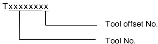
The 6-digit (or 7-digit) tool No. code data and start signal will be output to the PLC.
