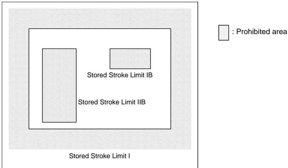
When an attempt is made to move the tool beyond the set range, an alarm is displayed, and the tool decelerates and stops. If the tool has entered into the prohibited area and an alarm has occurred, it is possible to move the tool only in the opposite direction to the direction in which the tool has just moved.
