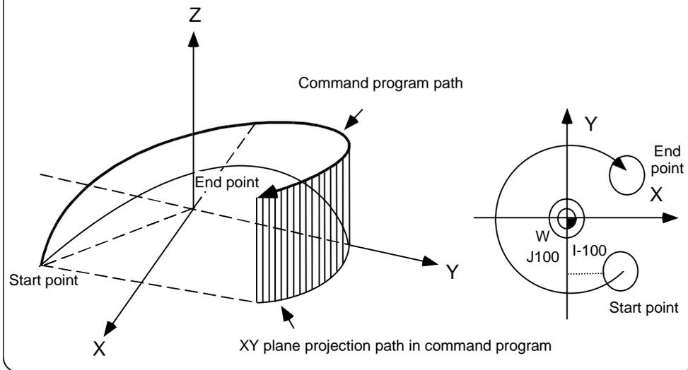
**(Note 1)** Helical sharps are machined by assigning linear commands for one axis which is not a circular interpolation axis using an orthogonal coordinate system. It is also possible to assign these commands to two or more axes which are not circular interpolation axes.
