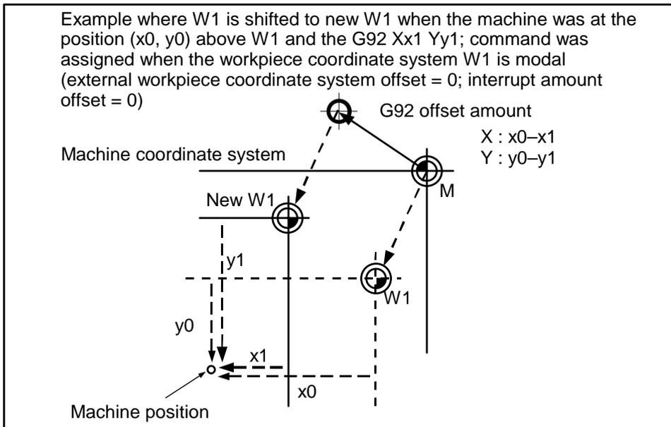
The shifted coordinate system is returned to its original position by dog-type reference position return or the program.
