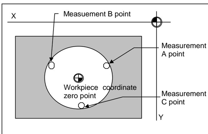
To set the workpiece coordinate offset, the position X and Y of the measurement A point are measured, and the measured values are set in the measurement A point. In the same manner as the measurement A point, the measurement B point and then C point are measured and set. The hole center coordinate is calculated by setting the workpiece coordinate system after setting three points, and the calculated result is set in the workpiece coordinate offset.
