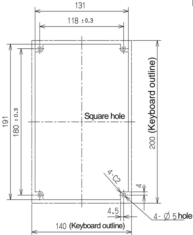
How to fix with screws from the back of the unit (Reference)
