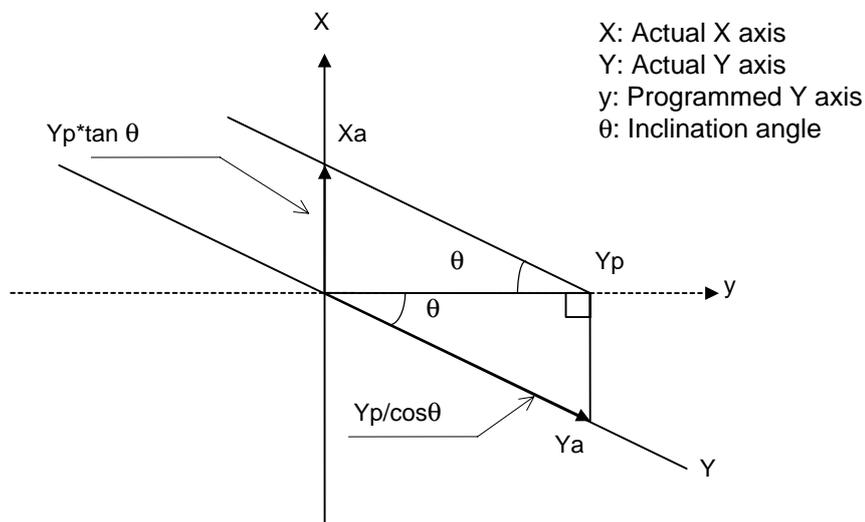
The Y-axis position and  $Y_p$  on the programmed coordinates (on the orthogonal coordinates) are respectively the  $X_a$  and  $Y_a$  positions produced by combining the X axis and Y axis along which the machine actually moves.
