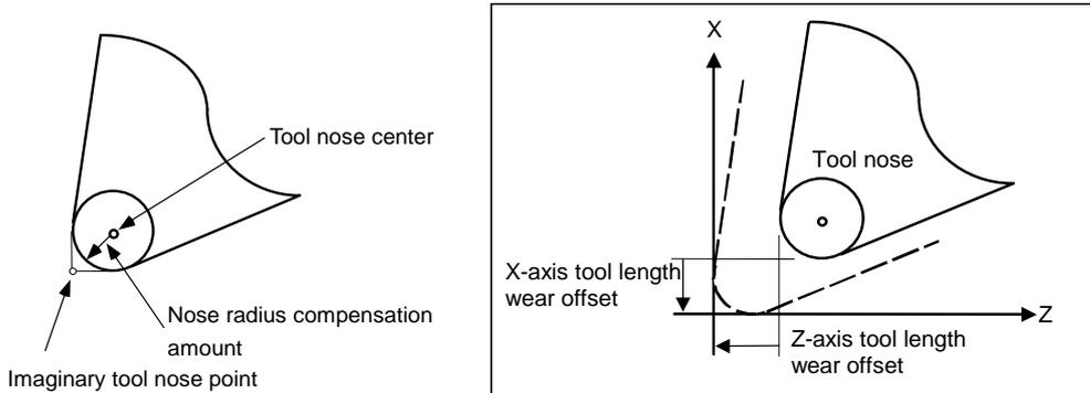
The X-axis tool length offset amount, Z-axis tool length offset amount and nose radius compensation amount are set as plus amounts.
