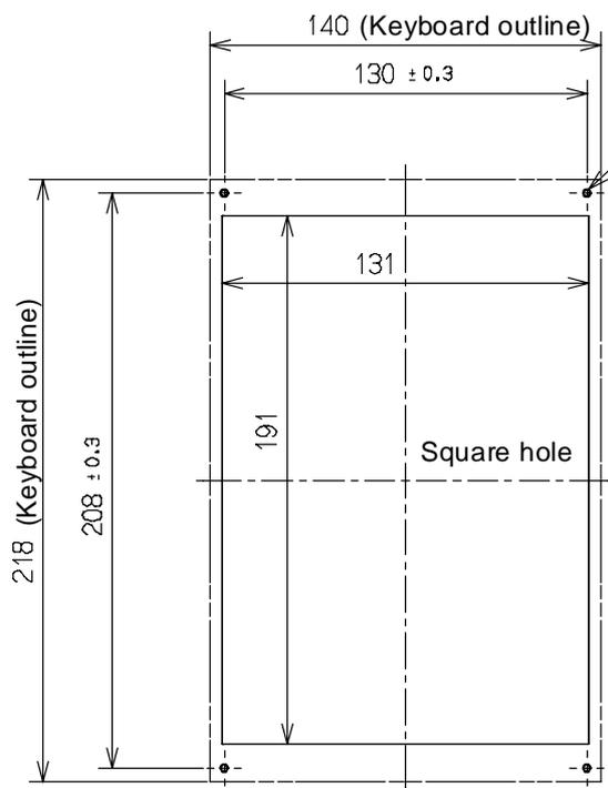
How to fix with screws from the front of the unit
