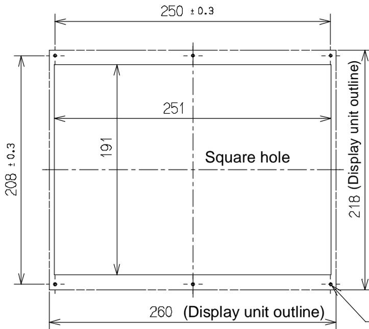
How to fix with screws from the front of the unit (Reference)
