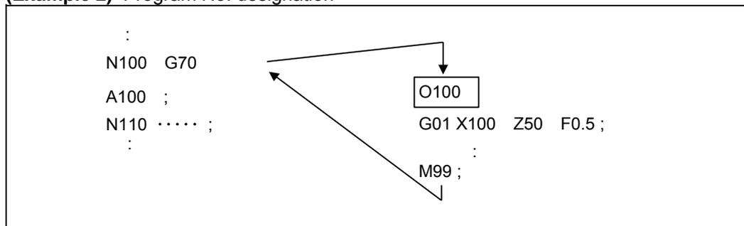
In either example 1 or 2, after the N100 cycle is executed, the N110 block is executed.
