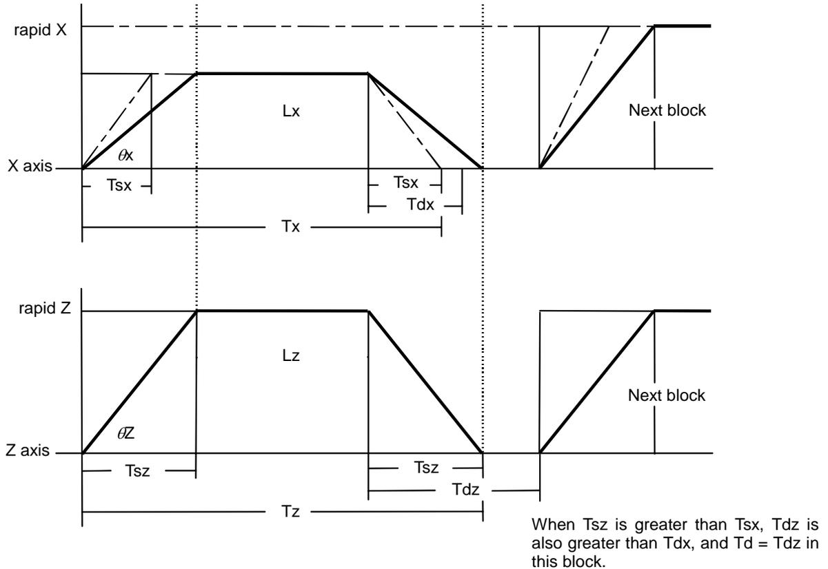
The program format of G0 (rapid traverse command) when rapid traverse constant inclination acceleration/deceleration are executed is the same as when this function is invalid (time constant acceleration/deceleration).
