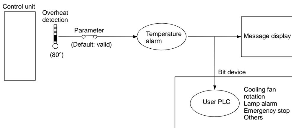
**(Note 1)** If the parameter is used to set the temperature rise detection function to invalid, overheating may occur, thereby disabling control and possibly resulting in the axes running out of control, which in turn may result in machine damage and/or bodily injury or destruction of the unit. It is for this reason that the detection function is normally left "valid" for operation.
