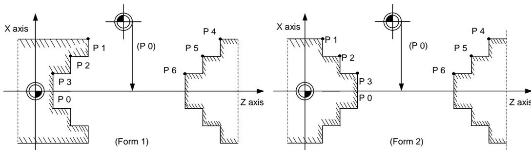
The chuck barrier and tail stock barrier are both set with the machine coordinate by inputting one set of three-point data in the parameter. Points P1, P2 and P3 are the chuck barrier, and points P4, P5 and P6 are the tail stock barrier. The X axis is set with the coordinate value (radius value) from the workpiece center, and the Z axis is set with the basic machine coordinate system coordinate.
