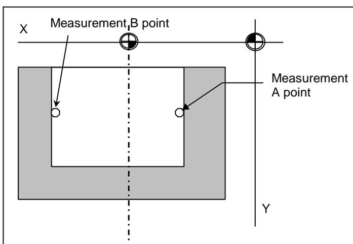
To set the workpiece coordinate offset, the position X (position Y) of the measurement A point is measured, and the measured value is set in the measurement A point. In the same manner as the measurement A point, the measurement B point is measured and set. The groove width center coordinate of the X axis (Y axis) is calculated by setting the workpiece coordinate system after setting two points, and the calculated result is set in the workpiece coordinate offset.
