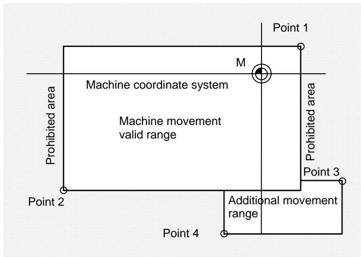
The position of points 3 and 4 are set with the machine coordinate.
