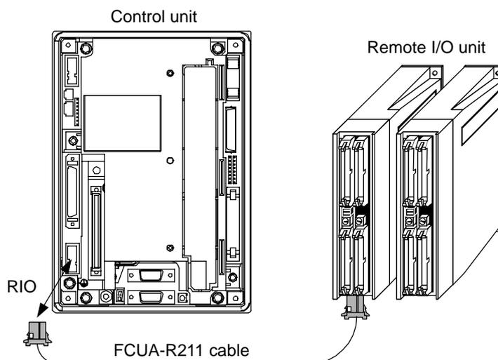
Assignment of the operation board remote I/O unit to the PLC device includes the following two patterns and can be switched.
