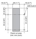
2) Mounting on the panel face Fit the Connector Conversion Box from the back side of the panel face, and fix it with four M3 screws (prepared by user). In the Connector Conversion Box, thread of M3, 6mm (0.23") in depth is cut in each mounting hole. Prepare four M3 mounting screws separately while con-sidering the thickness of the panel face.
