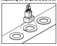
• Inspections for chips and burs on plastic molded parts.
