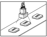
• Checks for IC orientation and front/back positioning.
