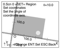
If the workpiece is on an angle, use the Down/Right and Up/Left Keys to specify the angle for the axis.
