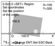
Align the origin of the coordinates (0) with the left corner or other part of the workpiece that will serve as the origin for the physical units.
