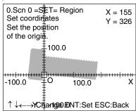
Align the origin of the coordinates (O) with the left corner or other part of the workpiece that will serve as the origin for the physical units.
