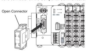
2. Open the terminal cover on the Screw Terminal Block Adapter and connect the cable conductors to BDH (communications data high signal) and to BDL (communications data low signal) on the terminal block. For Round Cable II, also connect BS+ (communications power supply +) and BS– (communications power supply –).
