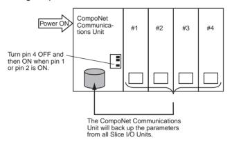
These conditions are necessary to back up the parameters. Do a check of these conditions before you back up the parameters.
