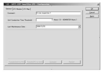
3. Click the **I/O Module** Tab and select the *Use Software Configuration Mode* Check Box. This will enable the Mount Check Boxes.
