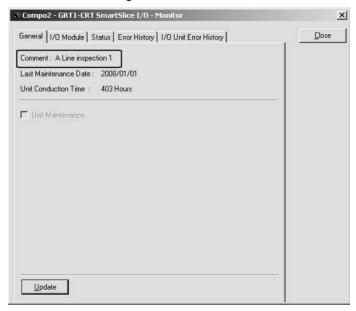
**Note** The comment shows by the icon of the CompoNet Communications Unit in the Maintenance Mode Window.
