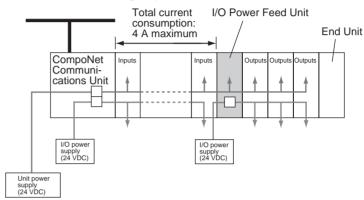
**Note** You can connect an I/O Power Feed Unit at the necessary location in the SmartSlice I/O Terminal to divide the input and output power supplies.
