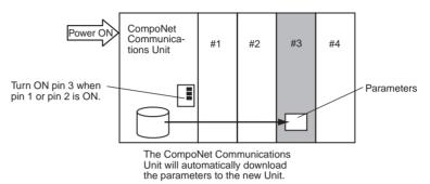
These conditions are necessary to automatically restore the parameters. Do a check of these conditions before you restore the parameters.
