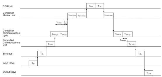
T<sub>IN</sub>: ON (OFF) delay time for Input Unit
