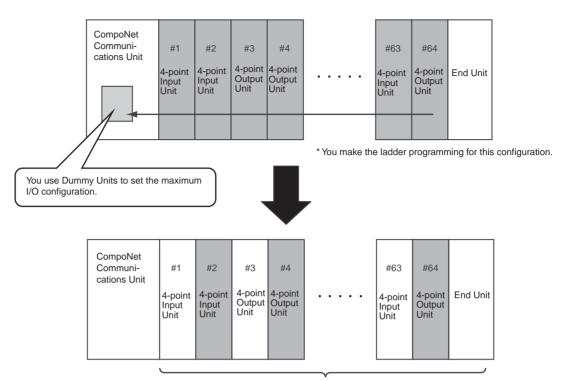
You replace Dummy Units with Slice I/O Units as the Slice I/O Units become necessary.
