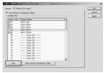
The Configuration Window will be displayed for the selected Unit. Refer to the *GRT1 Series SmartSlice I/O Units Operation Manual* (Cat. No. W455) for information the parameters.
