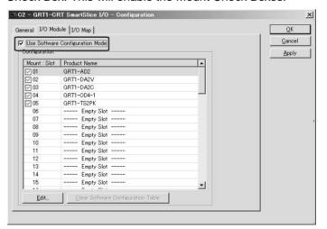
4. Select the *Mount* Check Boxes for all SmartSlice I/O Units in the Smart-Slice I/O Terminal and clear the *Mount* Check Boxes for all Dummy Units.
