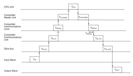
T<sub>IN</sub>: ON (OFF) delay time for Input Unit
