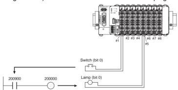
**Note** The figure below shows the allocations of I/O bits in the CPU Unit to the SmartSlice I/O Terminal.
