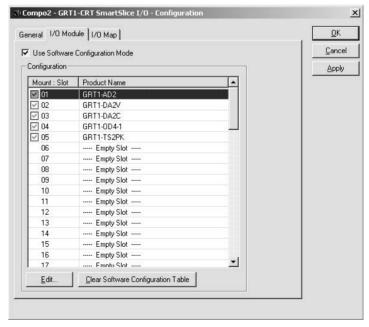
The CompoNet Communications Unit will clear the Software Setting Table.
