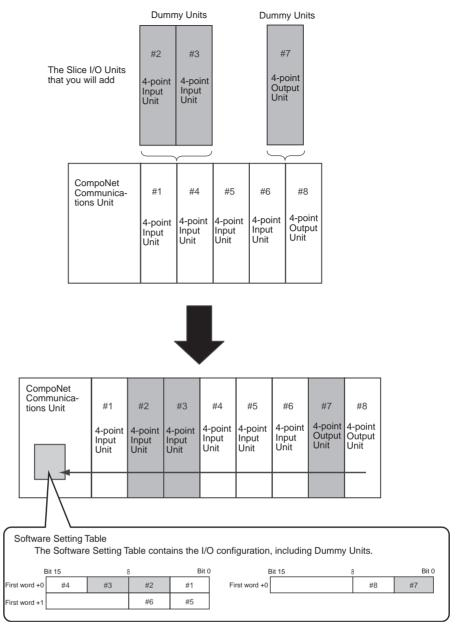
You can set Dummy Units to make the I/O configuration information and ladder programming for the maximum configuration. This will decrease the effects of changes in the SmartSlice I/O Unit configuration on the I/O configuration information and ladder programming.
