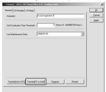
4. Click the **Transfer [PC to Unit]** Button. The CX-Integrator will download the Software Setting Table to the CompoNet Communications Unit.
