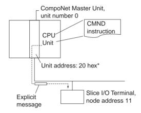
\*The unit address of the CompoNet Master Unit (a Special I/O Unit) is the unit number plus 20 hex.
