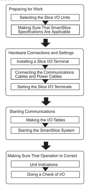
Note This example tells you the most basic setting and application procedures. For information on other settings which are necessary for system operation, refer to the CS/CJ-series CompoNet Master Unit Operation Manual (Cat. No. W456) and the GRT1 Series SmartSlice I/O Units Operation Manual (Cat. No. W455).
