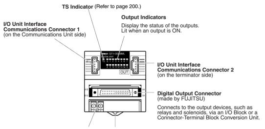
Terminal Block DIN Track Mounting Hook
