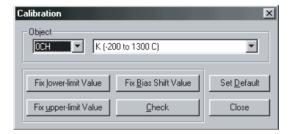
The calibrated upper limit will be stored in the EEPROM in the Temperature Input Unit.
