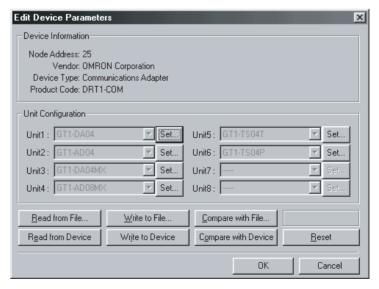
The specified output range and output for communications errors will be set for the Analog Output Unit. At this stage, however, the setting is not enabled.
