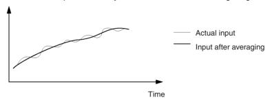
**Note** The time required for refreshing converted data remains 1 ms/point when the averaging function is enabled. The first communications data after the power is turned ON will be output after averaging eight samples.
