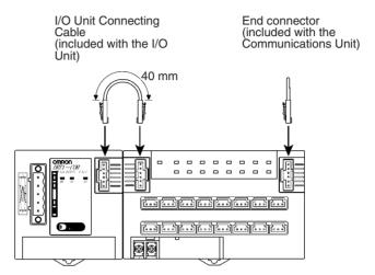
Connect the I/O Units in order, in the way shown in the above diagram. A maximum of 8 Units can be connected.
