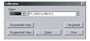
The calibrated lower limit will be stored in the EEPROM in the Temperature Input Unit.
