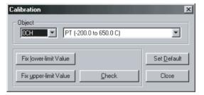
8. Calibrate the lower limit. Apply18  $\Omega$  to the input terminal (as selected in step 7) on the Temperature Input Unit from the 6-dial precision resistance box. Wait approximately 1 minute for the input to stabilize, then click *Fix lower-limit Value*.
