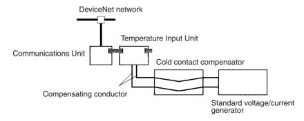
Use a calibrated thermocouple in the cold junction compensator and a compensating conductor, and set the cold junction compensator to 0°C.
