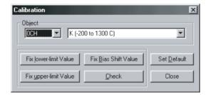
The calibrated lower limit will be stored in the EEPROM in the Temperature Input Unit.
