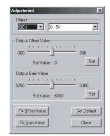
11. Click *Fix Gain Value* when the voltage output or current output is correct for 100%.
