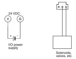
Note V terminals and V connector pins, as well as G terminals and G connector pins, are internally connected. When the I/O power is being supplied from a terminal block, the power can be supplied to the output devices from the V and G connectors. Current supplied in this way, however, must be less than 2 A.
