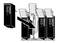
3. When the Relay has been pushed inside as far as it will go, raise the lever so that it is covering the top of the Relay.
