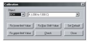
8. Calibrate the lower limit. Apply 0 mV to the input terminal (as selected in step 7) on the Temperature Input Unit from the standard voltage/current generator. Wait approximately 1 minute for the input to stabilize, then click *Fix lower-limit Value*.
