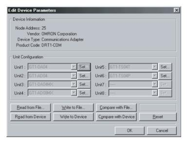
The specified input ranges will be set in the Temperature Input Unit. At this stage, however, the settings are not enabled.
