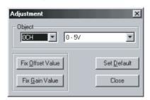
The gain will be adjusted so that the input voltage or input current will be converted to a value of 100%, and the value of the gain will be stored in the EEPROM in the Analog Input Unit. Reset the Unit to enable the new setting.
