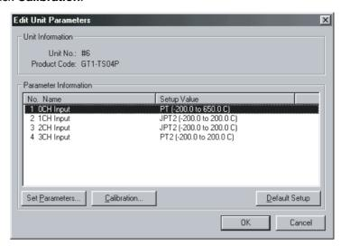
The Calibrate Unit Window will be displayed. At this time, the GT1-TS04P will enter Calibration Mode. While in Calibration Mode, temperature data sent to the Master will be 7FFF Hex. (7FFFFFF Hex if in 2-decimal-place Mode). Exit the Calibration Mode by resetting the MULTIPLE I/O TERMINAL, or by turning the power OFF and ON again, to return to normal operating conditions.
