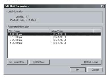
The Calibrate Unit Window will be displayed. At this time, the GT1-TS04T will enter Calibration Mode. While in Calibration Mode, temperature data sent to the Master will be 7FFF Hex. (7FFFFFF Hex if in 2–decimal-place Mode). Exit the Calibration Mode by resetting the MULTIPLE I/O TERMINAL, or by turning the power OFF and ON again, to return to normal operating conditions.
