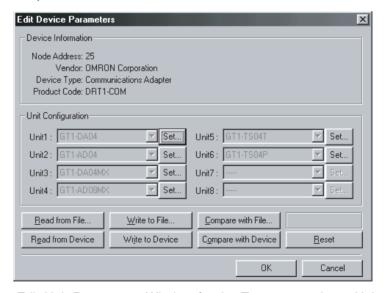
The Edit Unit Parameters Window for the Temperature Input Unit will be displayed.
