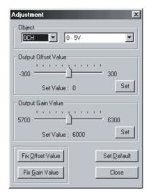
The offset value set using the slider bar will be stored in the EEPROM in the Analog Output Unit. Reset the Unit to enable the new setting.
