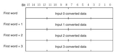
If the converted data is a negative number, it is stored as a two's complement. Data for range codes that include one digit after the decimal point are stored without the decimal point, i.e., 10 times the actual value is stored. Some examples are provided in the following table.
