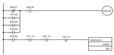
If any of the following occur after the Counter Unit setting and start-up have been completed (and 232.04 is ON), the Step Advance Bit 233.00 turns ON in order to reset the settings for the Counter Unit.
