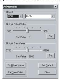
The voltage output or current output will be output on the output terminal on the Analog Output Unit designated in step 7. Adjust the slider bar until the output is correct for 0%.
