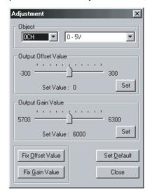
The voltage output or current output will be output on the output terminal on the Analog Output Unit designated in step 7. Adjust the slider bar until the output is correct for 100%.
