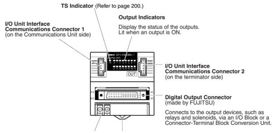
**Terminal Block DIN Track Mounting Hook**
