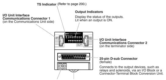
Terminal Block DIN Track Mounting Hook
