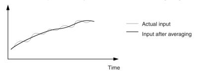
**Note** The time required for refreshing converted data remains one ms/point when the averaging function is enabled. The first communications data after the power is turned ON will be output after averaging eight samples.
