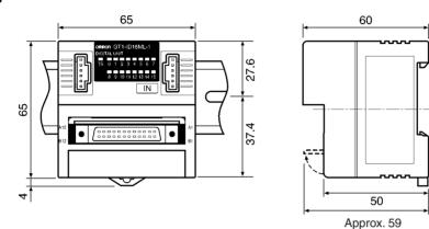
**Note** The vertical center of the Unit is 4.9 mm lower than the center of the DIN track. The Unit therefore extends downward 41.4 mm (including the mounting hook) from the DIN track center.
