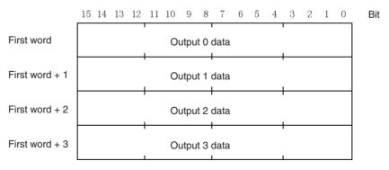
When a negative voltage is to be output, specify the conversion data as the two's complement. To obtain a two's complement from an absolute value, the NEG instruction is useful.
