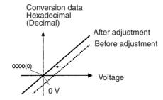
The possible range of offset adjustment depends on the input range. Refer to the following table.
