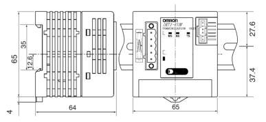
**Note** The vertical center of the Unit is 4.9 mm lower than the center of the DIN track. The Unit therefore extends downward 41.4 mm (including the mounting hook) from the DIN track center.
