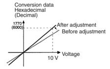
The possible range of gain adjustment depends on the input range. Refer to the following table.
