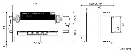
**Note** The vertical center of the Unit is 4.9 mm lower than the center of the DIN track. The Unit therefore extends downward 41.4 mm (including the mounting hook) from the DIN track center.
