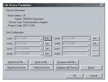
The specified input range will be set for the Analog Input Unit. At this stage, however, the setting is not enabled.
