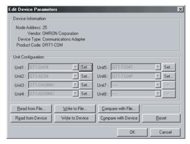
The Communications Unit and all the I/O Units connected to the Communications Unit will be reset, and the specified parameters (for example, for input range) will be enabled.
