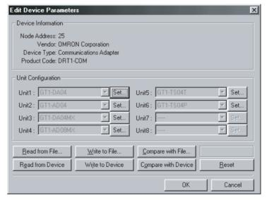
The Communications Unit and all the I/O Units connected to the Communications Unit will be reset, and the specified parameters (for example, for input ranges) will be enabled.
