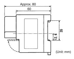
**Note** The vertical center of the Unit is 4.9 mm lower than the center of the DIN track. The Unit therefore extends downward 41.4 mm (including the mounting hook) from the DIN track center.
