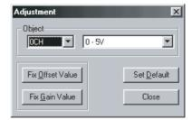
The offset will be set so that the input voltage or input current are converted to a value of 0%, and the value of the offset will be stored in the EEPROM in the Analog Input Unit. Reset the Unit to enable the new setting.
