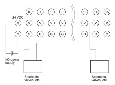
**Note** V terminals and G terminals are internally connected. When the I/O power is being supplied, the power can be supplied to the output devices from the V terminals and G terminals. Current supplied in this way, however, must be less than 4 A.
