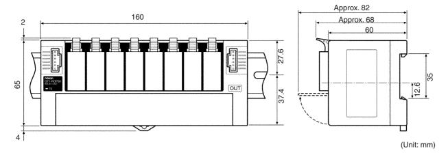
**Note** The vertical center of the Unit is 4.9 mm lower than the center of the DIN track. The Unit therefore extends downward 41.4 mm (including the mounting hook) from the DIN track center.
