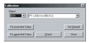
The calibrated upper limit will be stored in the EEPROM in the Temperature Input Unit.
