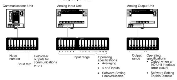
Note a) If a DeviceNet Configurator (versions 1.11 and later) is used, the input range for Analog Input Units, the output range for Analog Output Units, and I/O Unit interface error output (high-clear output/low-clear output) can be set via the network. When setting from the Configurator, use the DIP switch to set the Software Setting Enable/Disable setting to Enable. For details, refer to 5-1 Analog Input Units and 5-2 Analog Output Units.
