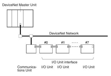
Checking the I/O Unit Interface Status
