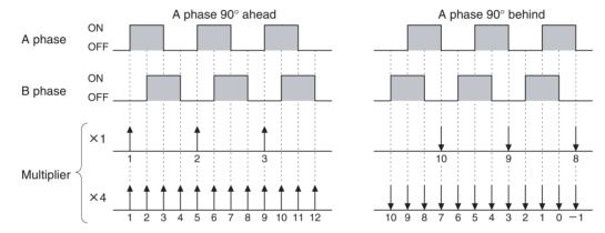
**Note** When using differential phase pulse input at a multiple function setting of  $\times 4$ , the count number for each revolution of the encoder will be 4 times the resolution of the encoder. Use an encoder that is compatible with the counting range.
