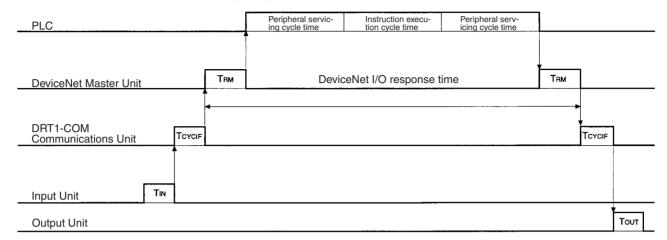
T<sub>IN</sub>: Input I/O Unit ON (OFF) delay time
