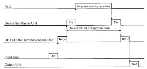
T<sub>IN</sub>: Input I/O Unit ON (OFF) delay time
