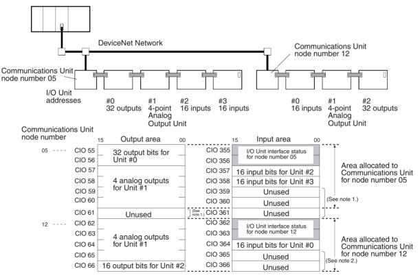
Note 1. The unused words between I/O areas that are used cannot be used as work bits.
