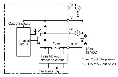
Note When the fuse blows, the F indicator lights and bit 08 turns ON. Bits 08 through 15 cannot be used as IR bits.
