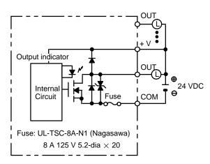
Note 1. No blown fuse detector circuit is provided.
