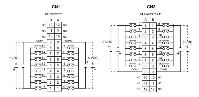
**Note** 1. I/O word "n" is determined by the unit number setting (n = IR  $100 + 10 \times \text{unit number}$ ).
