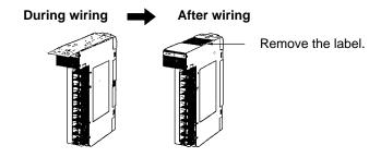
Wire the Units so that they can be easily replaced. In addition, make sure that the I/O indicators are not affected by the wiring.
