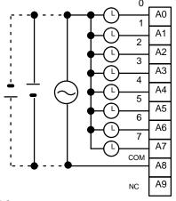
250 VAC 24 VDC max. (inductive load: 2 A resistive load: 2 A) (8 A/Unit)
