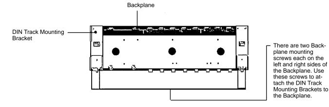
2. Mount the Backplane to the DIN Track so that the claws on the Mounting Brackets fit into the upper portion of the DIN Track as shown below.
