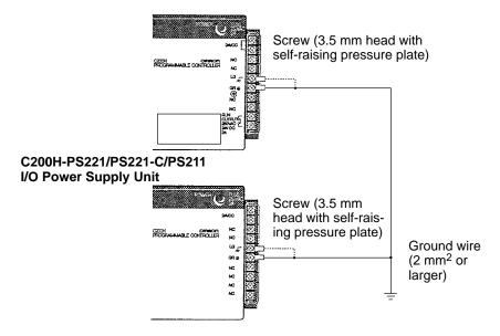
**Note** The LG terminal is not provided for the C200HS-CPU01-EC CPU and C200H-PS221-C I/O Power Supply Unit.
