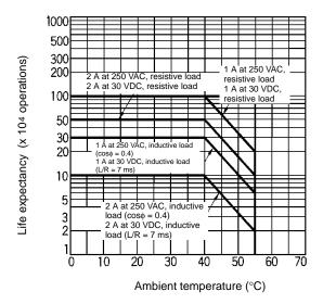
**Note** 1. If the Contact Output Unit is panel-mounted, the temperature inside the panel represents the ambient temperature.
