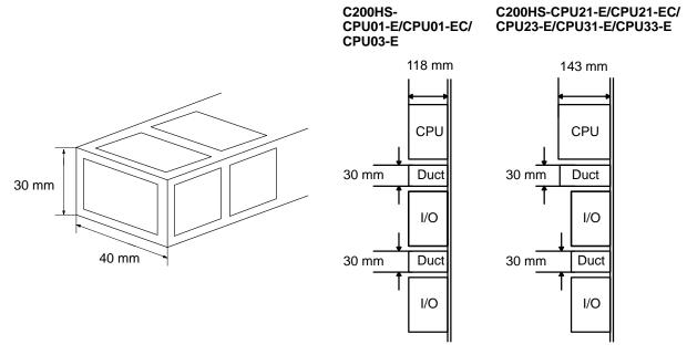
Each Rack must be mounted vertically, that is, with the printing on the front panels oriented as it would normally read. Racks may be directly mounted to any sturdy support meeting the environmental specifications.
