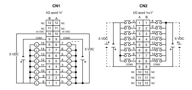
**Note** 1. I/O word "n" is determined by the unit number setting (n = IR 100 + 10  $\times$  unit number).
