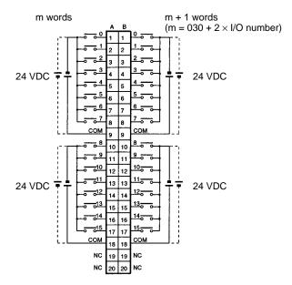
**Note** 1. The polarity of the input power supply can be either positive or negative. The polarity of all commons, however, must be the same.
