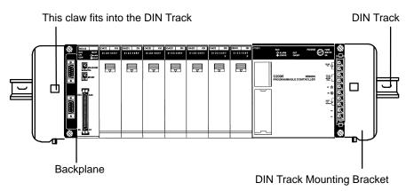
3. Loosen the screws attaching the Mounting Brackets to the Backplane. Slide the Backplane upward as shown below so that the Mounting Bracket and Backplane clamp securely onto the DIN Track. Tighten the screws.
