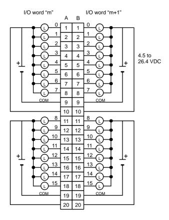
**Note** 1. I/O word "m" is determined by the I/O number setting (m = IR 030 +  $2 \times I/O$  number).
