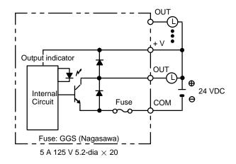
Note 1. No blown fuse detector circuit is provided.
