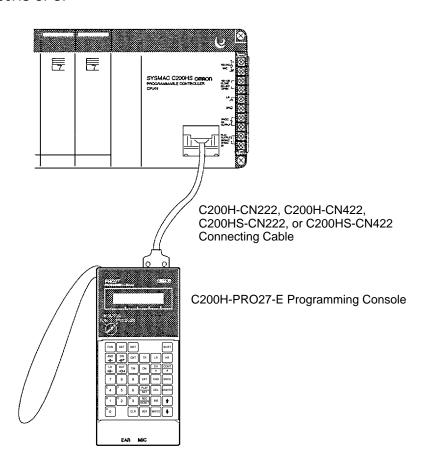
As indicated in the illustration, the C200H-PRO27-E Programming Console connects to the C200HS CPU with C200H-CN222, C200H-CN422, C200HS-CN222, or C200HS-CN422 Connecting Cable which must be purchased separately. The C200HS-CN222 and C200HS-CN422 Connecting Cables conform to EC directives.
