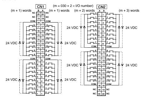
**Note** 1. The polarity of the input power supply can be either positive or negative. The polarity of all commons for CN1 and CN2, however, must be the same.
