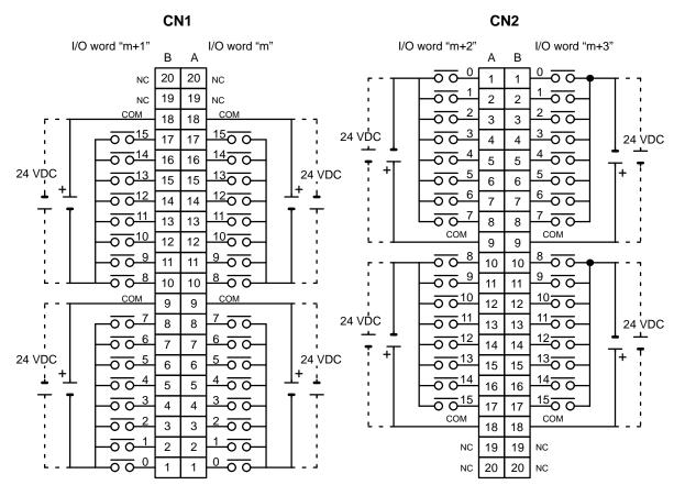
**Note** 1. I/O word "m" is determined by the I/O number setting (m = IR 030 +  $2 \times I/O$  number).
