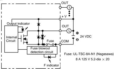
Note When the fuse blows, the F indicator lights and bit 08 turns ON. Bits 08 through 15 cannot be used as IR bits.
