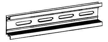
DIN Track Mounting Bracket The DIN Track Mounting Bracket shown below is necessary for mounting the PC to the DIN Track.
