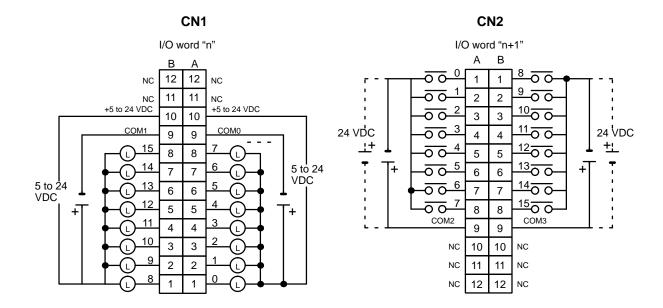
**Note** 1. I/O word "n" is determined by the unit number setting (n = IR  $100 + 10 \times \text{unit number}$ ).
