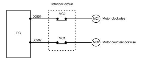
This circuit prevents outputs MC1 and MC2 from ever both being ON at the same time. Even if the PC is programmed improperly or malfunctions, the motor is protected.
