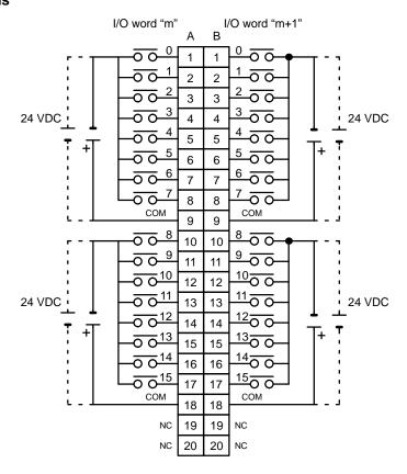
**Note** 1. I/O word "m" is determined by the I/O number setting (m = IR 030 +  $2 \times I/O$  number).
