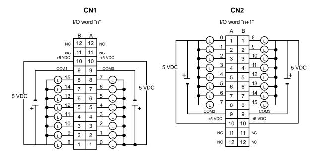
**Note** 1. I/O word "n" is determined by the unit number setting ( $n = IR 100 + 10 \times unit number$ ).
