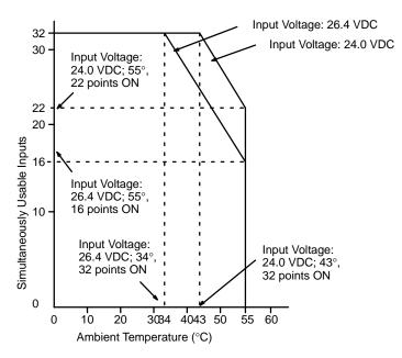
**Note** If the Unit is at room temperature it takes about 10 minutes for excessive heat to build up when all inputs are turned ON, so all inputs can be turned ON simultaneously for testing.
