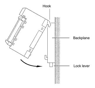
Press down on the yellow lock lever at the bottom of the slot, press the I/O Unit firmly into position, and then release the yellow lock lever.
