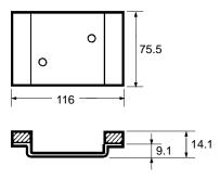
Take the space required for the cable into consideration when mounting the Programming Console to panels.
