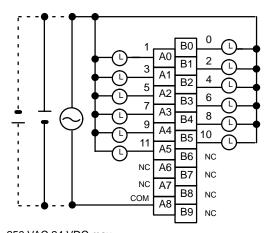
250 VAC 24 VDC max. (inductive load: 2 A resistive load: 2 A) (8 A/Unit)
