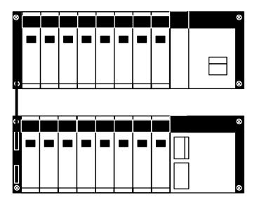
The CPU Rack and Expansion I/O Rack shown above are connected by a Connecting Cable (the length of Cable between individual Racks can be up to 10 m, but the total length of Cable between all Racks must be within 12 m).
