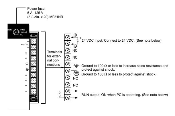
**Note** Use a 24-VDC power supply with reinforced insulation or double insulation if the EC directives (low-voltage directives) must be satisfied.
