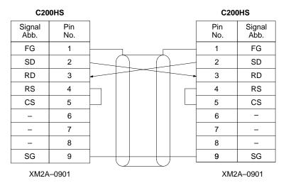
Ground the FG terminals of C200HS Units at a resistance of less than 100  $\Omega$ .
