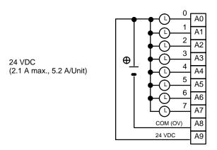
**Note** Be sure to supply power to A9; otherwise current will leak through the load while the output is OFF.
