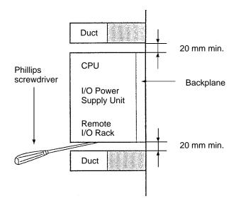
The mounting height of CPU Racks, Expansion I/O Racks, or Slave Racks is 118 mm or 143 mm depending on the type of I/O Units mounted. If Peripheral Devices or connection cables are attached, the additional dimensions must be taken into account. Allow sufficient clearance in the control panel in which the PC is mounted.
