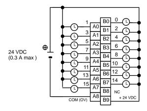
Note 1. Be sure to supply power to B9; otherwise current will leak through the load while the output is OFF.
