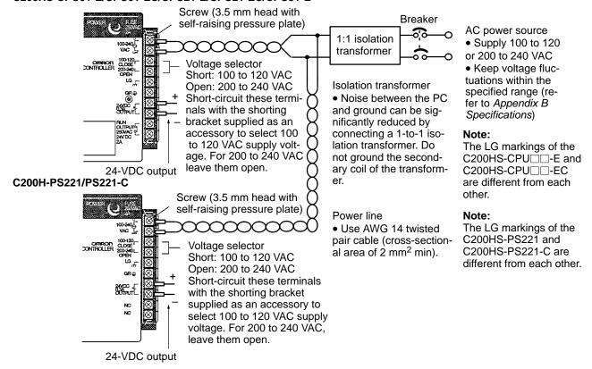
**Note** The C200HS-CPU01-EC CPU, C200HS-CPU21-EC CPU, and C200H-PS221-C I/O Power Supply Unit do not have an LG terminal.
