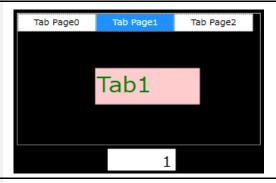
8. When you switch the tabs using the variable, if you enter a value outside the specified range, no tab page will be displayed. Make sure to specify the upper and lower limits for the Data Edit object to avoid entry of any value outside the range.
