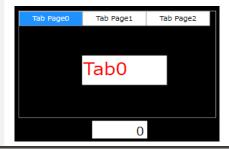
5. Check the operation of switching the tab by changing the value of the variable assigned to the Tab Control object.
