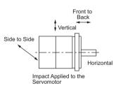
The servomotor will withstand the following vibration acceleration in three directions: vertical, side to side, and front to back.
