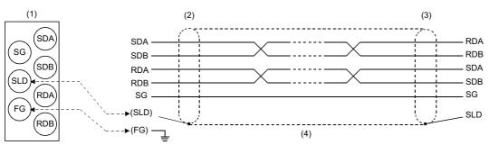
(1): Correspondence of the RS-422/485 terminal block and signal position
