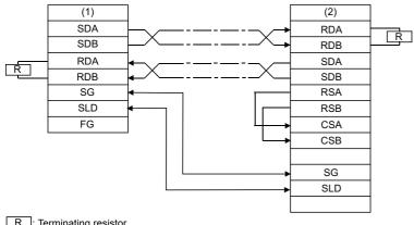
R: Terminating resistor (1): C24
