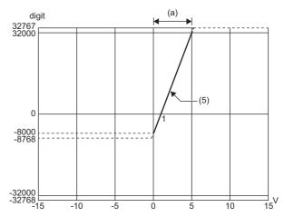
digit: Digital output value V: Analog input voltage (V)
