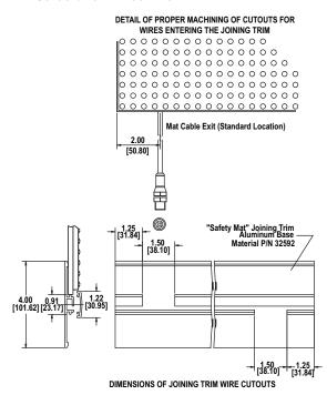
Figure 7-5 Joining Trim Wire Cutouts
