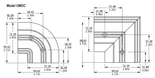
Figure 4-2 Dimensions and Installation Information for 2-Part Aluminum Base, PVC Cover with Molded Corners
