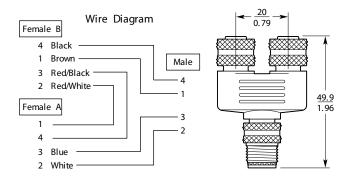
Figure 3-3 "Y" Connector Pinouts
