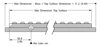
Mat Cable exits on the side indicated by the first dimension in the model number i.e. UM5-1254, Cable exits 12" dimension i.e. UM5-4824, Cable exits 48" dimension
