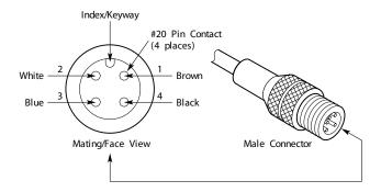
Figure 3-2 Cable Pin-outs
