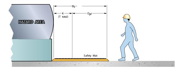
Figure 6-1 Safety Mounting Distance
