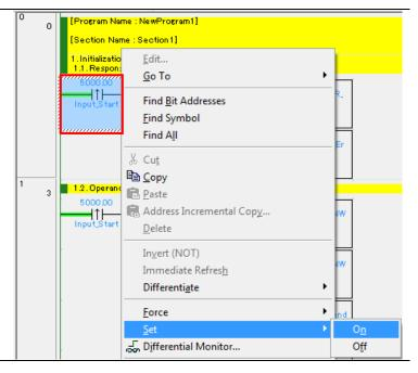
4 Confirm that the *Input\_Start* contact is turned ON as shown in the right figure.
