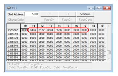
\* The data display can be changed from hexadecimal to text by selecting **Display** - **Text** from the View Menu.
