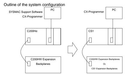
The table below lists the models of SYSMAC $\alpha$  series units and each corresponding models of CS1-series. Select the CS1-series model which is compatible with the C200H Series model. Or, select the CS1-series model with similar specification to the C200H Series Unit.
