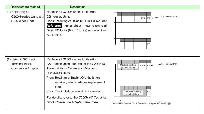
Note 1. Depending on the type of Basic I/O Unit, there may be some restrictions (e.g. change in I/O specifications or wiring) or some models cannot be used.
