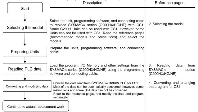
2) Actual replacement work: Take the steps below to replace the SYSMAC $\alpha$  series (C200HX/HG/HE) to CS1.
