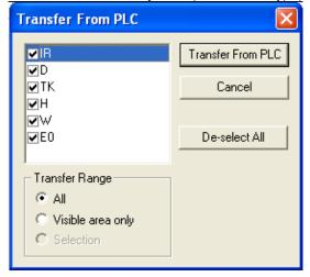
Scroll and check all the areas. Press the *Transfer from PLC* button to start loading.
