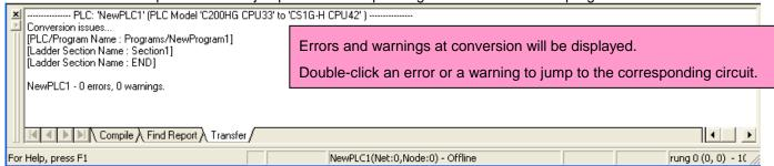
Some instructions can not be converted. Modify the ladder program by refferring to *Appendix A. Instructions* converted by Change Model on CX-Programmer.
