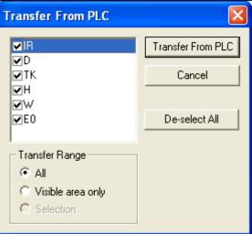
Scroll and check all the areas. Press the Transfer from PLC button to start transfer.
