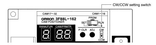
Set the direction of increasing angles to "CW" for clockwise direction when viewed from the Resolver axis, and "CCW" for counterclockwise direction (as shown in the following diagram).
