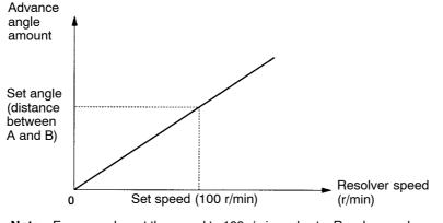
**Note** For example, set the speed to 100 r/min and set a Resolver angle corresponding to the distance between A and B as the set angle.
