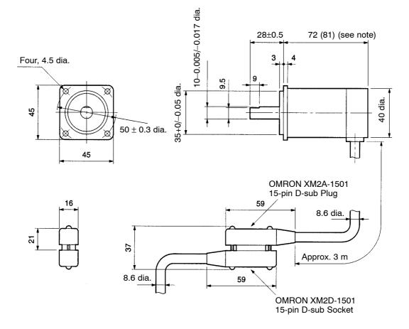
Note The dimensions in parentheses are for the 3F88L-RS17T Resolver.
