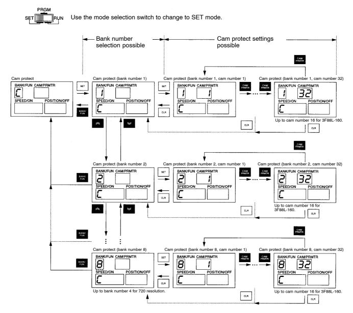
• Use the Bank/Function Key to set cam protect (Function No. C) and press the Set Key, and the bank number will flash in the Bank/Function display (indicating that bank number selection is enabled.)
