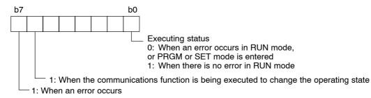
Bit 0 (executing status) is also set to 1 when the communications function is being executed to change the operating state (such as parameter settings) in RUN mode. For example, when the operating state is changed in RUN mode and there are no errors, "Status" will be set to "41."
