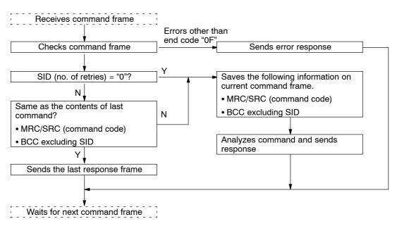
When initially sending a command frame, set SID to "0." If the corresponding response frame is abnormal, set SID to "1" and then resend the command frame.
