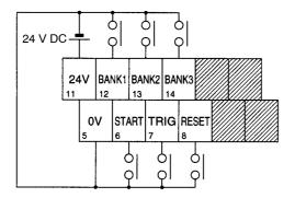
Terminal screw size: M3 Tightening torque: 0.5 N • m
