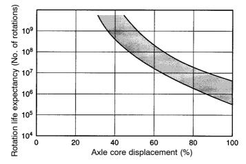
**Note** Axle core displacement is given as a percentage of allowable axle core displacement. (Refer to *2-2-3 Mounting the Resolver.*)
