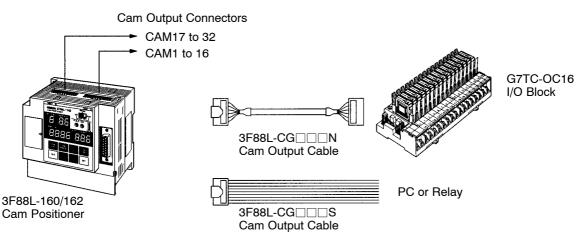
**Note** The 3F88L-160 16-output Cam Positioner does not have cam output connector terminal numbers CAM17 to CAM32.
