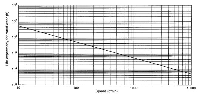
• 3F88L-RS15/RS15W Resolvers (Axle End Load: Radial and Thrust both 19.6 N)
