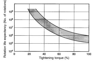
**Note** Tightening torque is given as a percentage of allowable tightening torque. (Refer to 2-2-3 Mounting the Resolver.)
