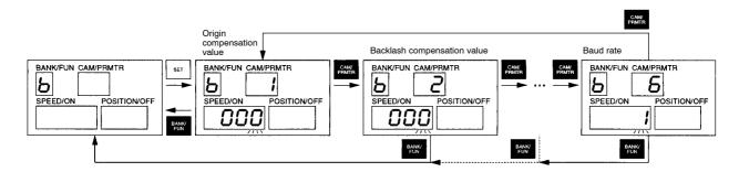
**Note** Set the function number (use the Bank/Function Key to change the function number and press the Set Key), display the parameter numbers, and then use the Cam/Parameter Key to set the parameter numbers (for functions with multiple parameter numbers). The parameter number will increase each time the Cam/Parameter Key is pressed. If the Cam/Parameter Key is pressed on the last parameter number (parameter number 6 in the above example), the display will return to parameter number 1.
