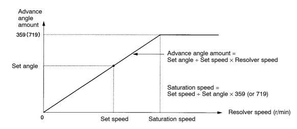
**Note** The maximum compensation value is 359 (for 360 resolution) or 719 (for 720 resolution). compensation greater than one rotation cannot be made.
