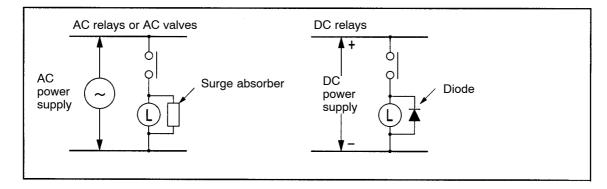
Note Select withstand pressure and current suitable for the load.
