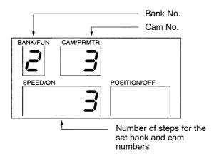
**Note** When the parameter number (PRMTR) is "0," the absolute angle for origin compensation is shown in the SPEED/ON display.
