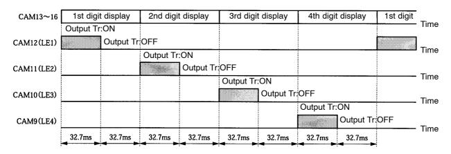
**Note** The output timing for each digit of display data (CAM 13 to 16) and each digit's LE signal (CAM9 to 12) are shown below.
