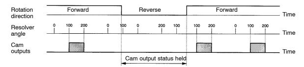
**Note** If both the one-direction function and the advance angle compensation function are set at the same time, cam outputs may be left out or output twice when the advance angle data is compensated. (Refer to *3-6-6 Advance Angle Compensation*.)
