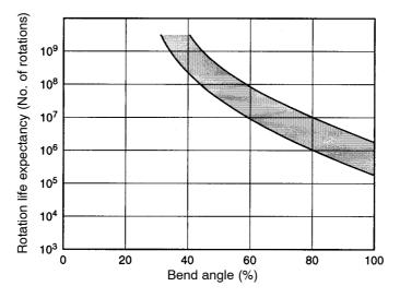
**Note** Bend angles are given as a percentage of allowable bend angles. (Refer to *2-2-3 Mounting the Resolver*.)
