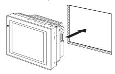
3. Secure the NSJ Controller to the panel using the enclosed Mounting Brackets. Tighten the Mounting Brackets evenly to the specified torque. Excessive tightening or insufficient tightening may deform the front sheet of the NSJ Controller.
