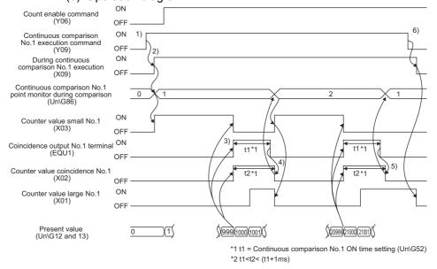
Figure 5.4 Operation example of the continuous comparison function
