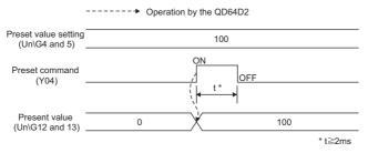
Figure 3.14 Operation of the preset command (Y04)
