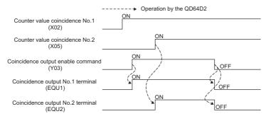
Figure 3.13 Operation of the coincidence output enable command (Y03)
