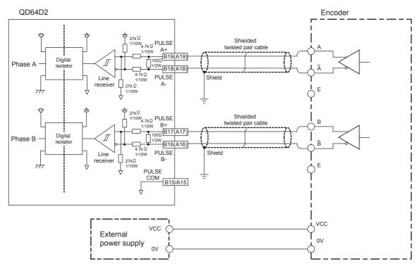
Figure 4.6 Example of wiring with a line driver (AM26LS31 equivalent) encoder
