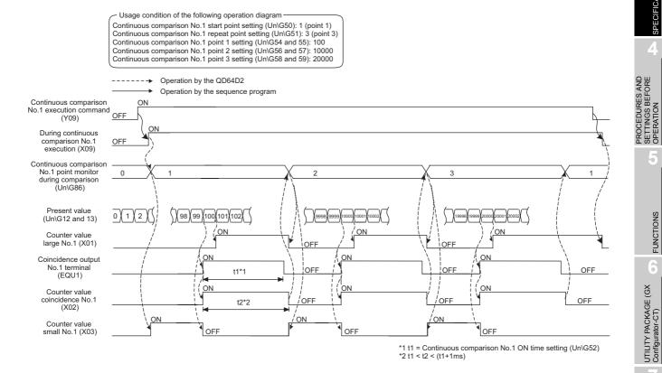
Figure 3.8 Operation of the counter value large No.1 (X01), the counter value coincidence No.1 (X02) and the counter value small No.1 (X03) when using the continuous comparison function
