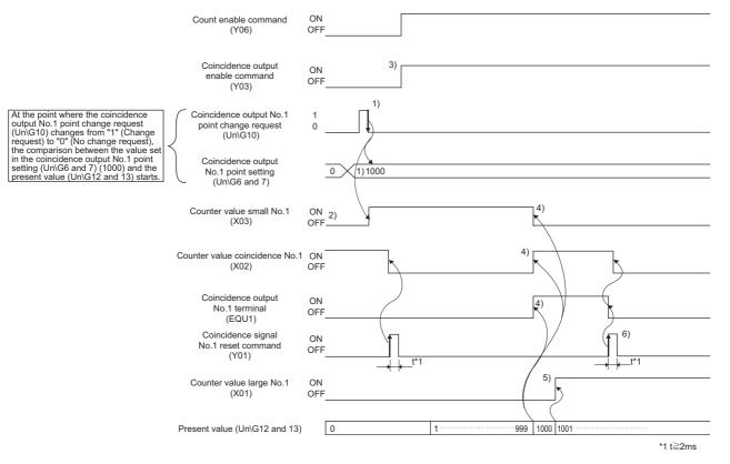
Figure 5.3 Operation example of the coincidence output function
