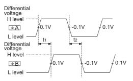
Figure 3.2 Pulse input waveform at 2-phase input 1
