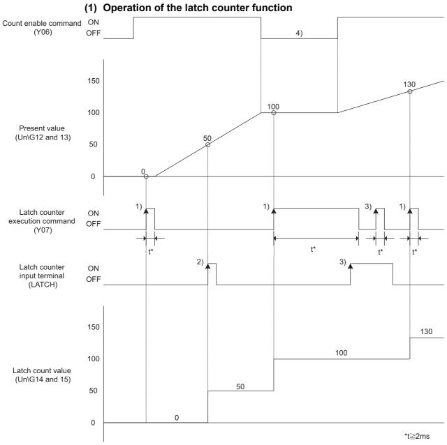
Figure 5.14 Operation example of the latch counter function
