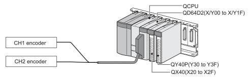
Figure 7.2 System configuration
