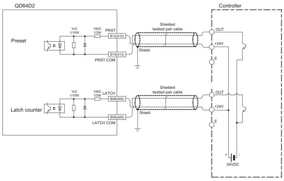
Figure 4.7 Example of wiring with a controller (sink loading type)
