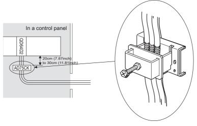
Figure 4.4 AD75CK cable clamp
