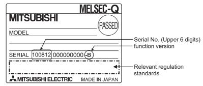
Figure 2.2 Checking the serial No. and function version (rating plate)
