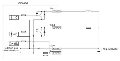
Figure 4.9 Example of wiring with an external output terminal (sink output type)
