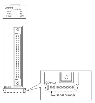
Figure 2.3 Display on the front of the module
