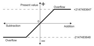
Figure 5.1 Operation image of the linear counter
