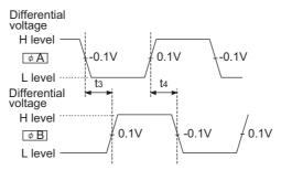
Figure 3.3 Pulse input waveform at 2-phase input 2
