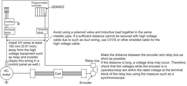
Figure 4.3 Example of wiring for measures against noise
