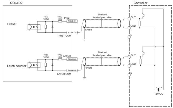
Figure 4.8 Example of wiring with a controller (source loading type)
