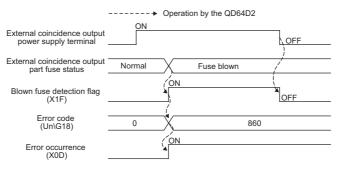
Figure 3.12 Operation of the blown fuse detection flag (X1F)
