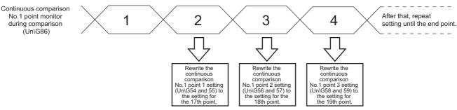
Figure 5.5 Rewriting data during comparison
