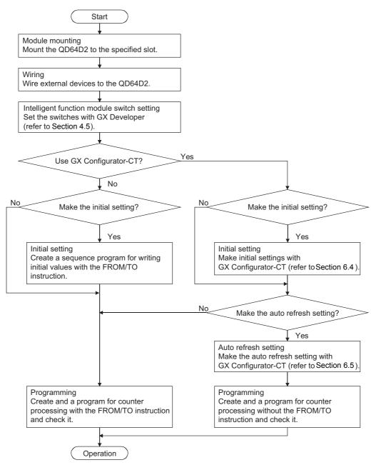
Figure 4.1 Procedures before operation
