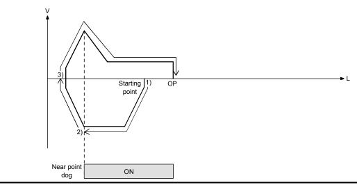
Fig. 8.13 OPR retry operation
