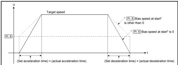
(Set acceleration/deceleration time) = (actual acceleration/deceleration time) if "Pr. 6 Bias speed at start" is either 0 or other than 0
