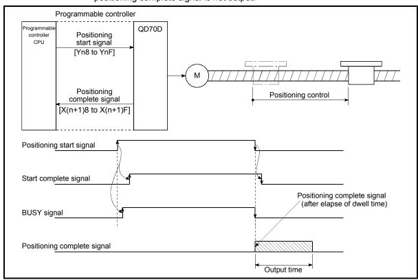
Fig. 4.2 Positioning complete signal output time
