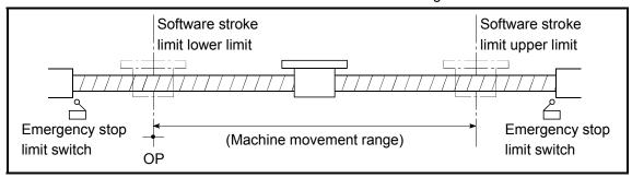
Fig. 4.1 Software stroke limit setting example
