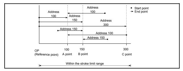
Fig. 9.5 Absolute system positioning control
