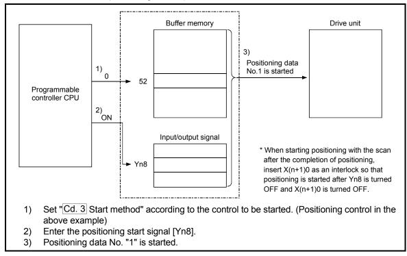
Fig. 7.2 Procedures for starting control (for axis 1)
