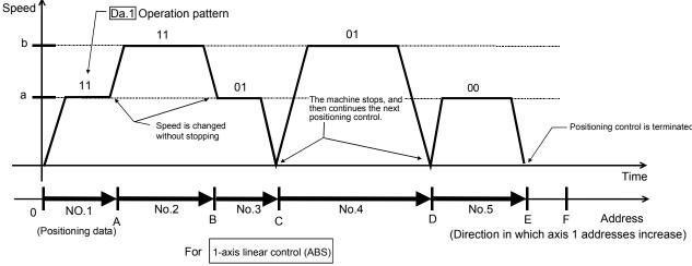
(One motor is driven, and positioning control is carried out to an addresses designated in one direction.)
