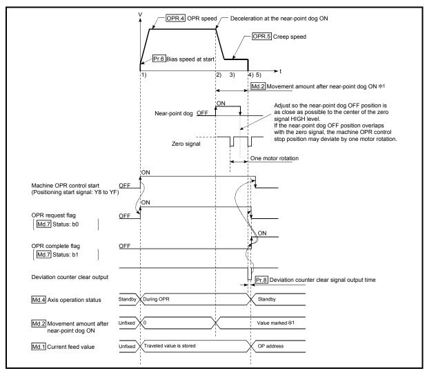
Fig. 8.2 Near-point dog method machine OPR control
