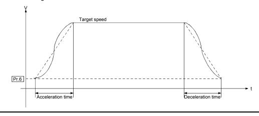
Fig. 11.7 Setting and operation of "Acceleration/Deceleration method"
