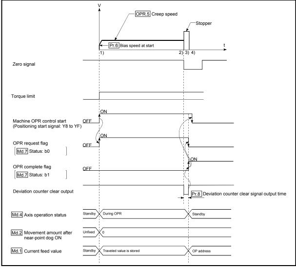
Fig. 8.8 Stopper 3 machine OPR control
