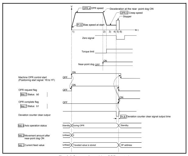
Fig. 8.6 Stopper 2 machine OPR control
