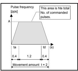
Fig. 1.1 Relationship between position control and speed control
