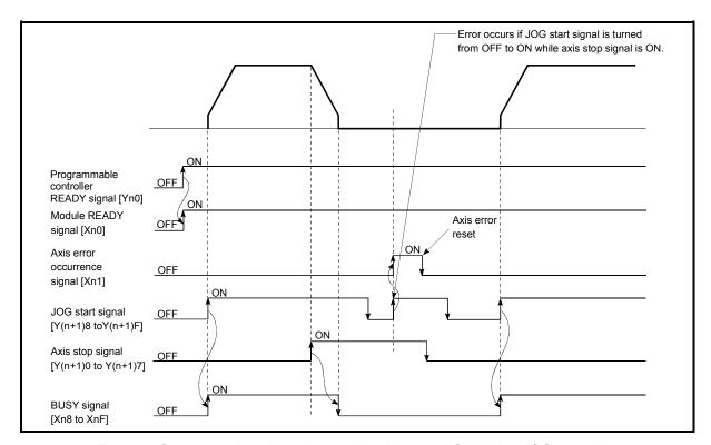
Fig. 10.2 Operation when the axis stop signal is turned ON during JOG operation
