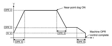
Pr. 6 Bias speed at start, OPR. 4 OPR speed, OPR. 5 Creep speed OPR. 6 ACC/DEC time at OPR, OPR. 7 DEC/STOP time at OPR
