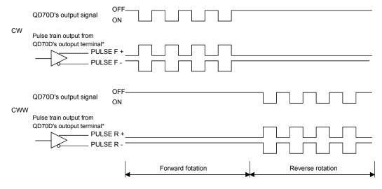
\*: PULSE F+/- and PULSE R+/- are waveforms based on PULSE F COM and PULSE R COM respectively.
