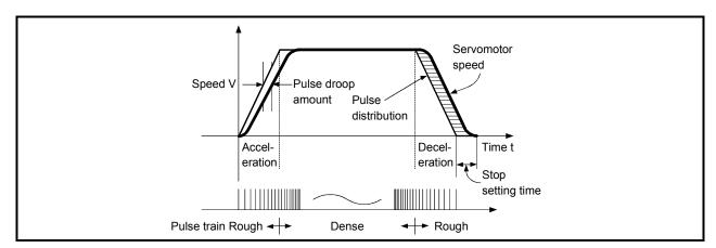
Fig. 1.3 QD70D output pulses
