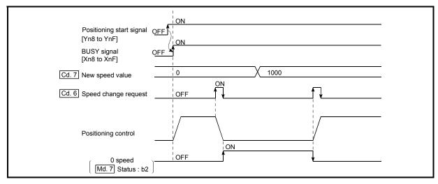
Fig. 11.3 Speed change at new speed value "0" (during speed control of speed-position switching control)
