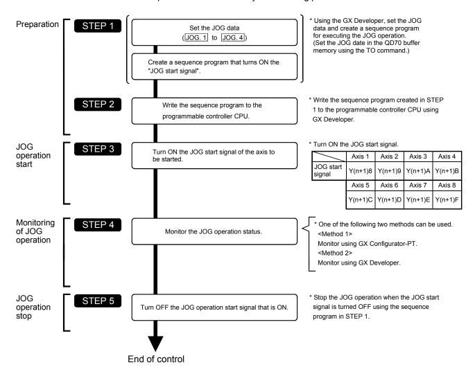
Refer to "Section 5.7 Simple reciprocating operation" for details of a JOG operation starting program.
