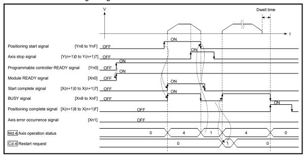
Fig. 7.10 Restarting timing chart (for position control)
