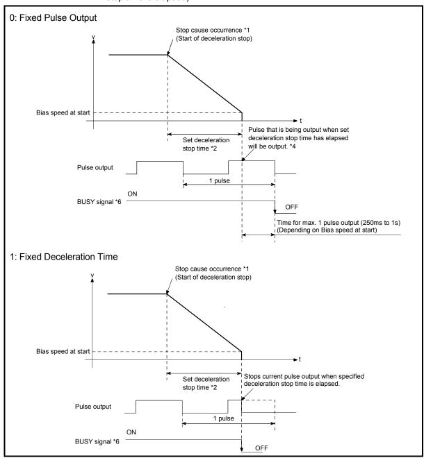
Fig. 4.7 Pulse output at deceleration stop
