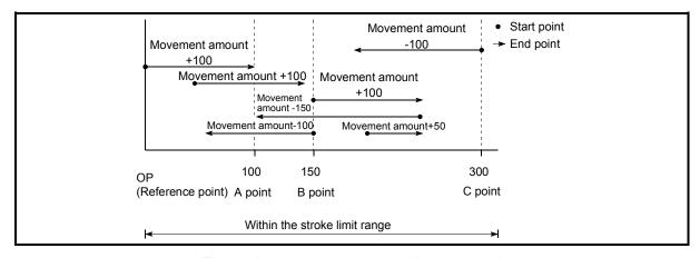
Fig. 9.6 Incremental system positioning control
