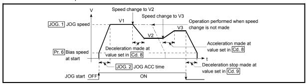
Fig. 11.1 Speed change operation
