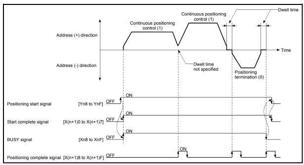
Fig. 9.2 Operation during continuous positioning control
