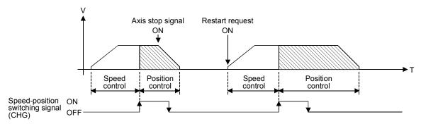
(b) When the speed-position switching signal (CHG) is ON at restart
