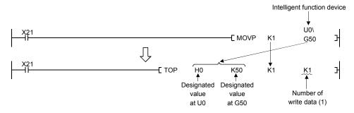
(b) When the circuit uses the "intelligent function device" on the source(s) side and the destination (D) side of a MOV command, change the command to a FROM command and a TO command.
