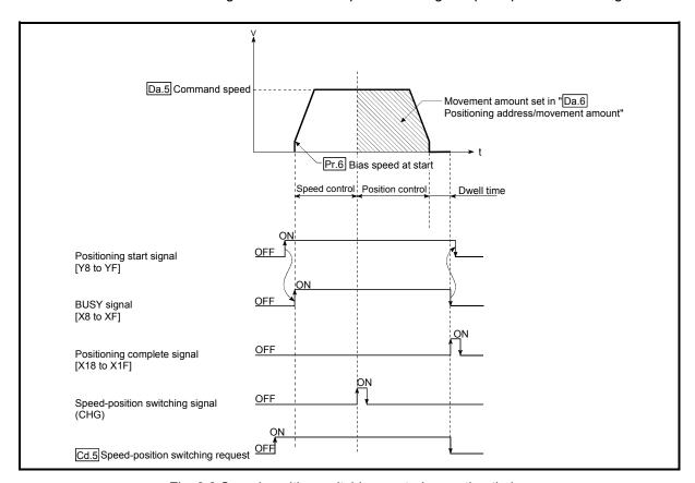
Fig. 9.8 Speed-position switching control operation timing
