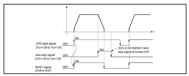
Fig. 10.5 Operation performed when axis stop signal is turned from ON to OFF with JOG start signal ON
