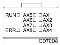
Each axis can be monitored by the states of the LEDs.
