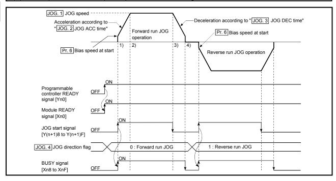
Fig. 10.1 JOG operation starting timing chart
