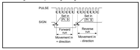
Fig. 4.3 PULSE/SIGN mode (set the pulse output mode with the intelligent function module switch. Refer to Section 5.6.)
