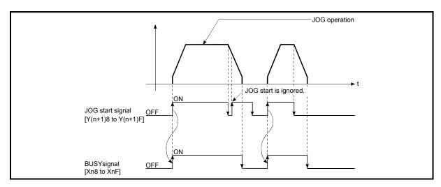
Fig. 10.4 Operation when the JOG start signal is turned ON during deceleration
