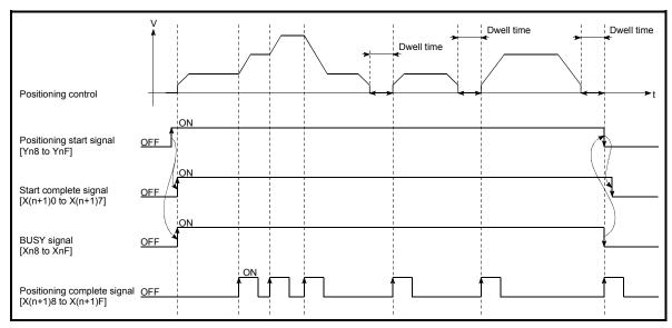
Fig. 7.3 ON/OFF timing of each signal at start of positioning control
