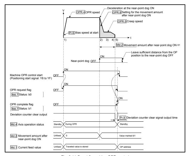
Fig. 8.11 Count 2 machine OPR control
