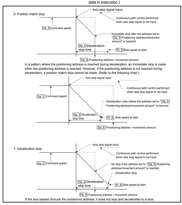
Fig.4.4 Deceleration stop by axis stop signal input
