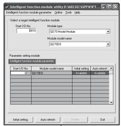
Refer to Section 6. 3. 3 Enter "Start I/O No.", and select "Module type" and "Module model name".
