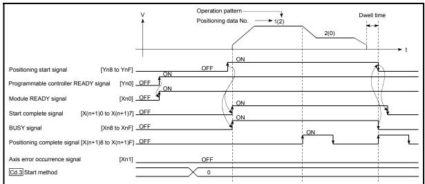
Fig. 7.6 Positioning control starting timing chart
