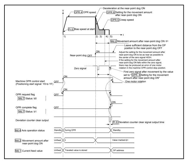
Fig. 8.10 Count 1 machine OPR control
