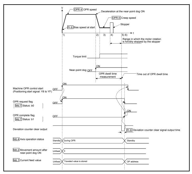
Fig. 8.4 Stopper 1 machine OPR control
