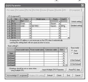
(a) I/O assignment setting screen Specify the following for the slot where the QD70D is mounted.
