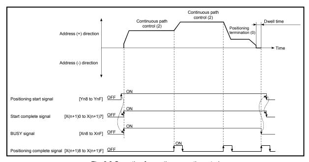
Fig. 9.3 Operation for continuous path control
