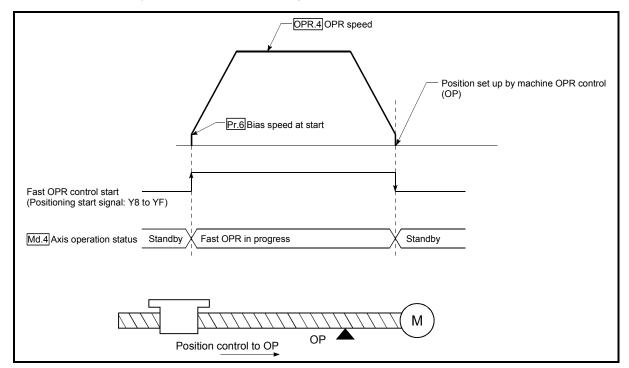
Fig. 8.12 Fast OPR control
