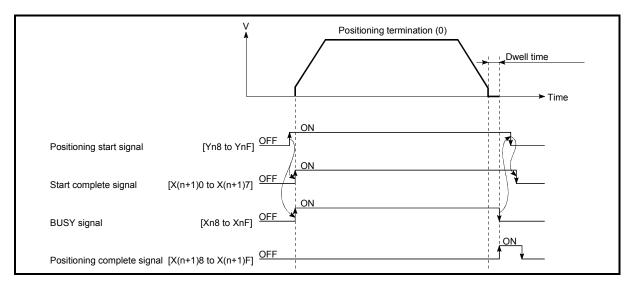
Fig. 9.1 Operation at positioning termination
