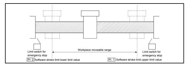
Fig. 11.5 Workpiece moveable range
