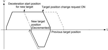
(3) When the target position change request is input, the work has started decelerating to stop.
