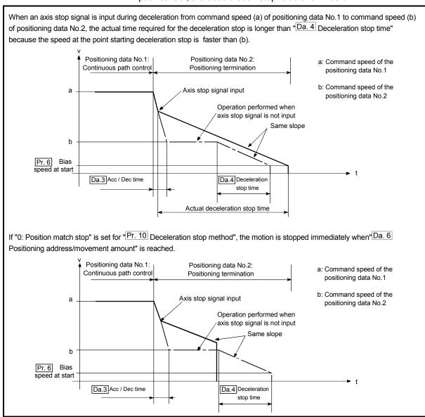
Fig.4.5 Deceleration stop when an axis stop signal is input during deceleration in continuous path control
