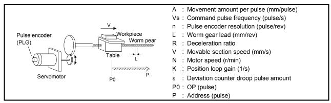
Fig. 1.4 System using worm gears
