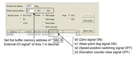
The states of the external I/O signals can also be checked by system monitor. For details, refer to "Section 12.3 External I/O signal monitor function".
