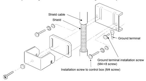
Using the AD75CK, you can tie four cables of about 7mm outside diameter together for grounding.
