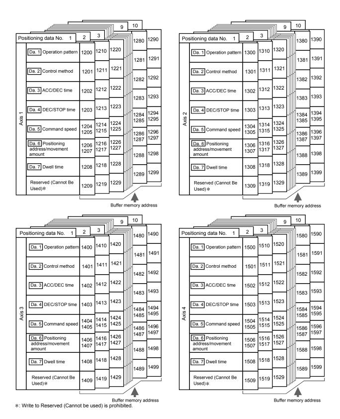
The descriptions that follow relate to the positioning data set items Da. 1 to Da. 7. (The buffer memory addresses shown are those of the "positioning data No. 1" for the axes 1 to 8.)
