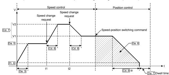
Pr. 6 Bias speed at start, Da. 3 ACC/DEC time, Da. 4 DEC/STOP time
