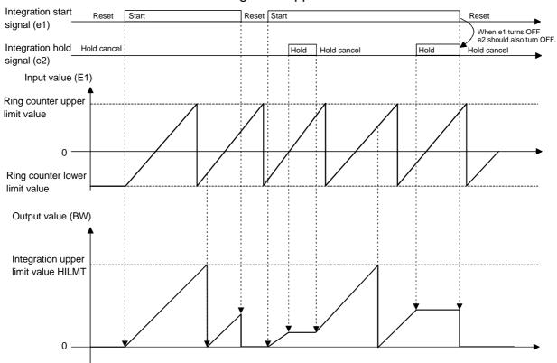
(1) Operation performed when the integration pattern is set to "integrated value returns to 0 when the integration upper limit value is exceeded"
