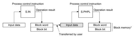
(3) The application of the input data changes depending on the used instruction. Refer to the explanation section of the corresponding instruction.
