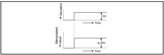
Fig. 1.3 Proportional operation when deviation is constant
