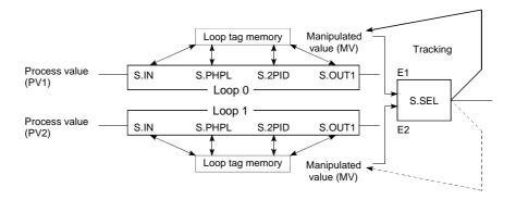
Example) When the S.SEL instruction uses the input value E1 and E1 uses the upper loop (loop 0) MV, the S.SEL instruction's MV is trucked to loop 0's MV. The setting that conducts Tracking is shown below.
