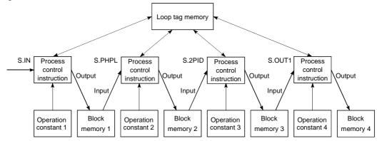
(b) Loop tag memory and operation constant locations in ladder diagram
