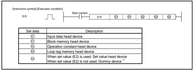
\*1: Special register SD1506 can be specified as a dummy device.
