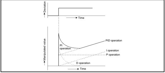
Fig. 1.6 PID operation when deviation is constant
