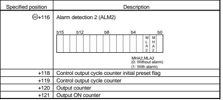
When control is to be started from the initial status, the data must be cleared with the sequence program.
