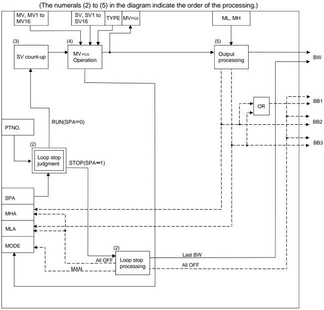
The processing block diagram of the S.PGS instruction is shown below. (The numerals (2) to (5) in the diagram indicate the order of the processing.)
