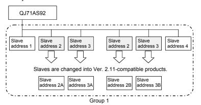
3) Prepare two QJ71AS92 modules. Then connect the slaves of the first and second systems to the respective modules.
