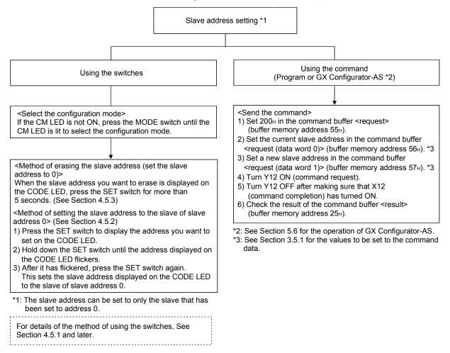
(2) Method of registering the configuration data to the QJ71AS92 Before starting operation in the protected operation mode, the configuration data of the slave that is ready for communication must be registered to the QJ71AS92.
