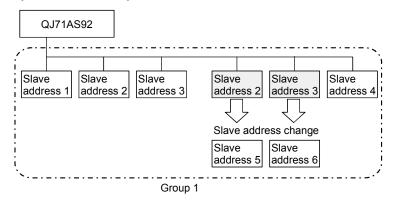
2) Change the slaves whose slave addresses overlap in the first and second systems into the AS-i Ver. 2.11-compatible slaves. Then split the slaves into two groups (A and B) and assign different slave addresses to group A and B, and connect the second system to the first system
