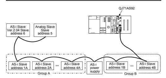
Use the AS-i cables, AS-i power supply and slaves that are compatible with AS-i Ver. 2.11 or AS-i Ver. 2.04.
