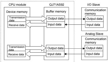
Automatic refresh at END processing of CPU module
