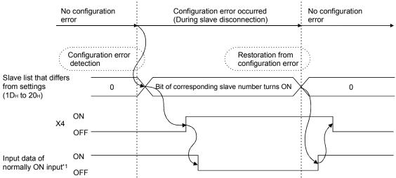
\*1: Shows the timing with the input data when the normally-ON input slave is disconnected.
