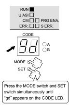
(2) Put the QJ71AS92 in the protected operation mode and register the configuration data of the slaves.
