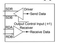
\*1 The "Output Control Input" (also called the send gate) of the driver (Send) portion in the figure at left decides whether data from SDA or SDB are output to an external device or not output.
