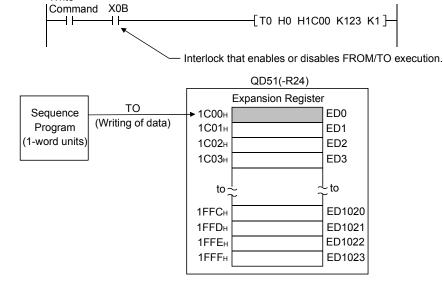
(2) During execution of a BASIC program by multitasking, data can be written or read from either task.
