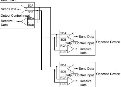
In the above wiring, sending and receiving are connected, the data sent by yourself is being received by yourself. Be sure to carry out programming so that such data are discarded by the BASIC program.
