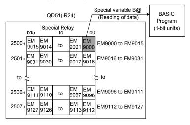
(b) Reading data by the FROM command in a sequence program
