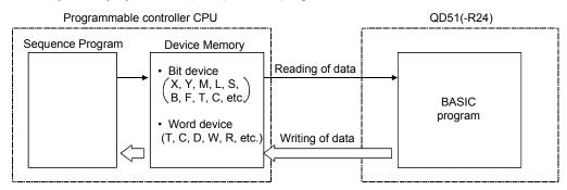
Refer to the Programming Manual (Commands) for the details of the device memories to and from which data can be written and read by the BASIC program.
