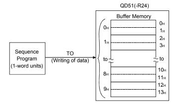
(b) In the QD51 (-R24), reading of data from, or writing of data to buffer memory is done using the GETMEM/PUTMEM command in the BASIC program.
