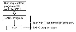
(b) For a task that is started by an interrupt from the programmable controller CPU, write it so that an "END" command is run at the end of the BASIC program.
