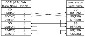
\* With the above wiring it is possible to carry out DC code control.
