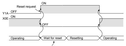
Reset after access enabled time (200/2000 ms) following the Y reset set by GX Developer.
