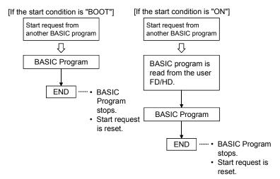
(b) For a task that is started by a start request from another BASIC program, write it so that an "END" command is run at the end of the BASIC program. If an "END" command is run, the start request is reset and it is made possible for the next interrupt to be received.
