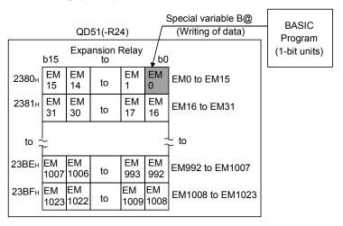
(b) In the FROM/TO command for writing or reading data in accordance with the FROM/TO command of a sequence program, an expansion relay is designated in the address. The designated address is in 1-word units, from 2380H to 23BFH.
