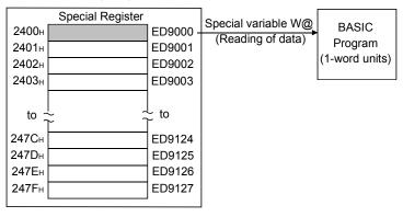
(b) Reading of data by the FROM command in a sequence program The special register is designated using the FROM command by the address.
