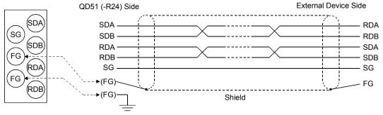
Correspondence between the RS-422/485 terminal block and signal positions
