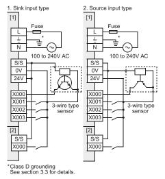
[1]:Main unit,Input/output extension unit (Common to both sink and source inputs)
