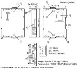
[1]FX3UC Main unit, FX2NC/FX3UC Extension block connector [2]FX3UC Main unit, FX2NC/FX3UC Extension block connecting hook
