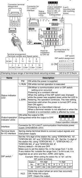
\* Set up using a slotted screwdriver with a tip width of 0.9 mm or less
