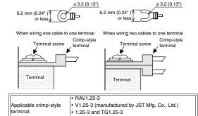
Applicable wire size 0.3 to 1.25 mm<sup>2</sup> Use a crimp-style terminal in a status in which no force is applied on the cable
