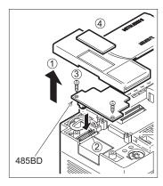
Turn off the power of the programmable controller, and mount the 485BD using the following procedure.
