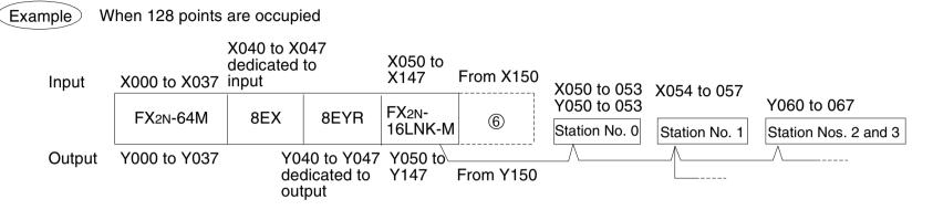
I/O assignment for remote I/O units
