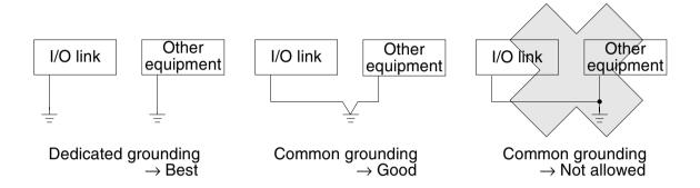
• When shielded twisted-pair cables are used, transmitted waveforms may be affected by the ground condition and communication errors may occur in a long-distance system.
