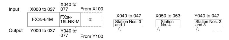
I/O assignment for remote I/O units
