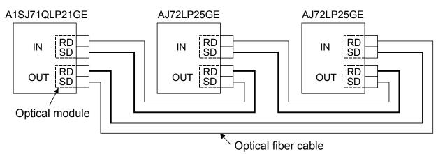
(3) When laying the optical fiber cable, do not touch the fiber core of the cable connector or module connector, or let dirt or dust collect on it.
