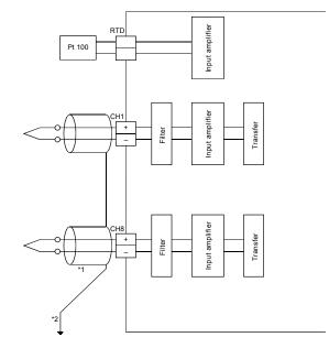
\*1 Be sure to use the shielded compensating conductor for the cable.
