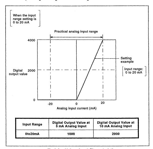
Fig 3.2 Volage Input Characteristics
