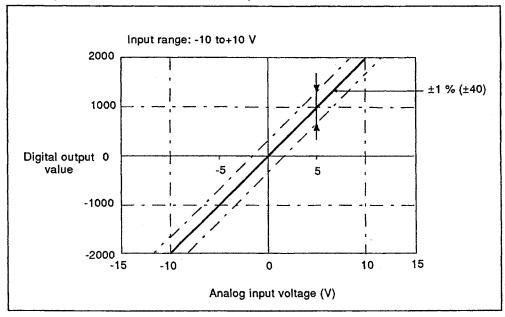
Fig 3.3 Overall Accuracy of the Voltage Input Characteristics
