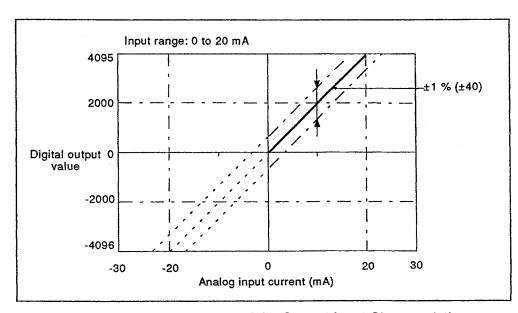
Fig 3.4 Overall Accuracy of the Current Input Characteristics
