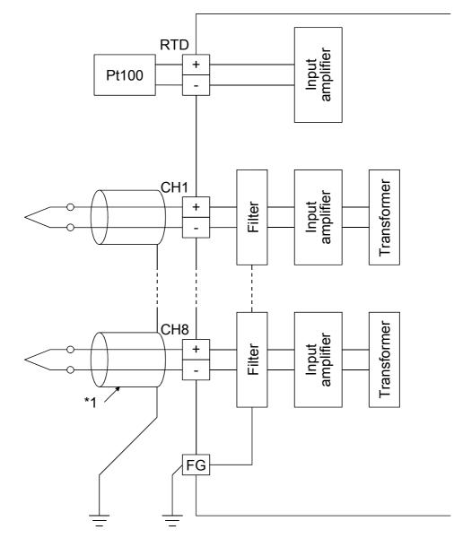
\*1: Use a shielded compensating conductor for the cable.
