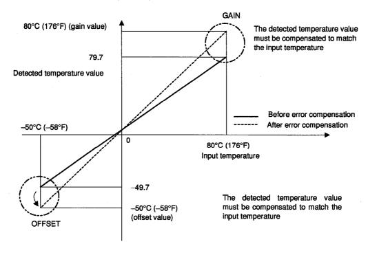
\* Error compensatoin can be done using a standard resistor instead of inputting a temperature directly to the Pt100.
