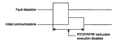
The following shows the faulty remote I/O station and detection timing during initial communications.
