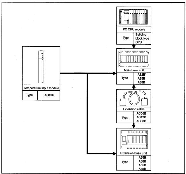
Fig. 2.1 Overall Configuration When a Building Block-Type CPU is used REMARK
