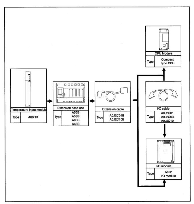
Fig. 2.2 Overall Configuration When a Compact-Type CPU is used
