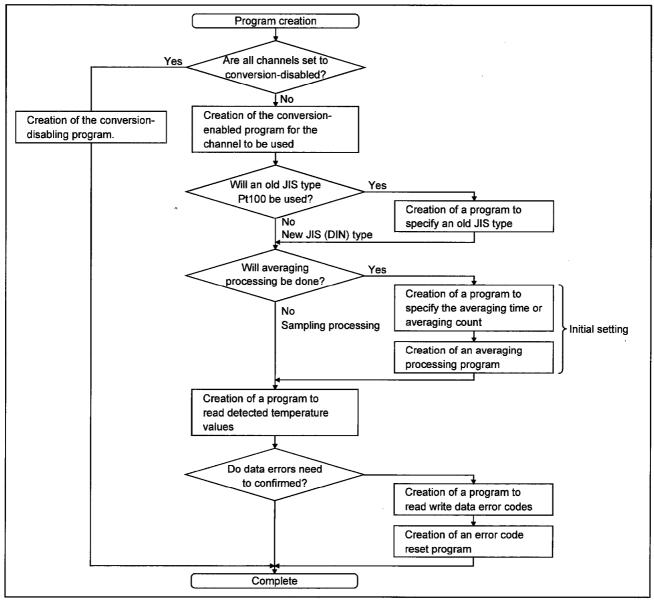
Fig. 5.1 Programming Procedure
