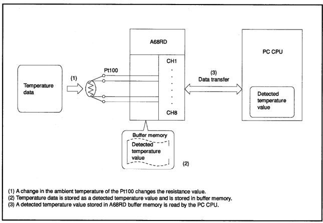
Fig. 1.1 Temperature Measuring Process
