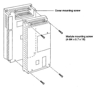
(2) Mounting the CPU module (or extension power supply module) to Type E56[ ][ ] I/O module
