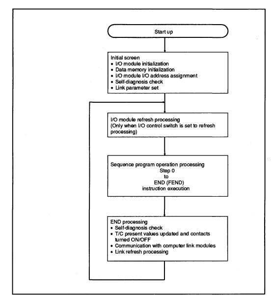
Fig. 4.1 A0J2HCPU Operation Processing
