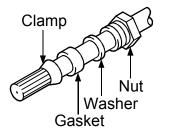
(c) Cut the external conductor, insulation material and internal conductor to the dimensions shown below. However, cut the external conductor to the same dimension as the tapered section of the clamp and smooth it down to the clamp.
