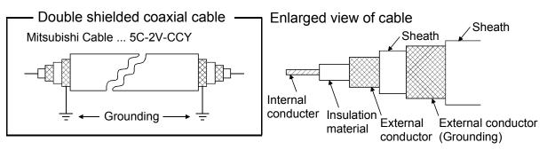
The 5C-2V connector plug is applicable to double-shielded coaxial cable. Connect the 5C-2V connector plug to the coaxial cable inside a double-shielded coaxial cable. Ground the shielded part outside a double-shielded coaxial cable as shown in the above figure.
