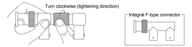
After connecting the F-type connector to the network module, retighten its ring periodically.
