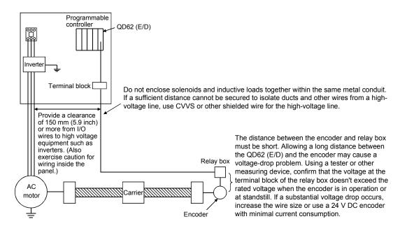
Grounding the shielded twisted pair cable is performed on the encoder side (relay box). (This example shows connection with 24 V sink load.
