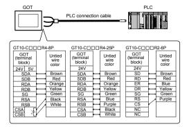
User-made cable is necessary, depending on the PLC. For the detail, refer to GOT1000 Series Connection Manual.
