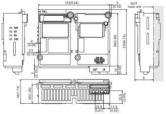
Dimensions of X when the CC-Link IE communication unit is mounted to the GOT.
