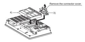
(5) Fix the CC-Link IE communication unit by tightening its mounting screws (4 places) with a tightening torgue of 0.36 to 0.48 N•m. (6) Fix the CC-Link IE communication unit by tightening two board fixing screws with a tightening torque of 0.36 to 0.48 N•m.
