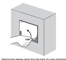
sheet. Do not remove the protective film. Position the sheet hole to the USB environmental protection cover on the GOT, and attach the sheet adhesive side.
