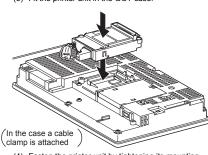
(4) Fasten the printer unit by tightening its mounting screws (2 places) with tightening torque 0.36 to 0.48
