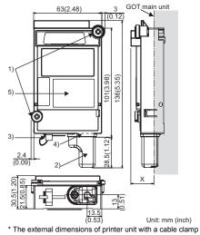
and connector holder attached is shown above
