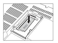
(5) After the installation of option function board, attach the extension unit cover. For installation of extension unit, install the extension unit
