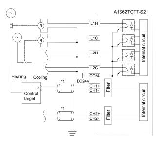
\*1: Always use the shielded compensating conductor for the cable.
