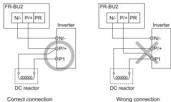
(6) When connecting several FR-BU2 to the inverter, be sure to connect terminal P/+, N/- of the FR-BU2 to terminal P/+, N/- of the inverter. Do not pass wires from terminal P/+ and N/- of the FR-BU2 to terminals of other brake unit.
