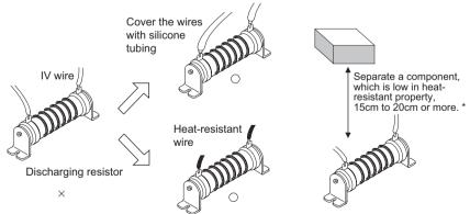
\* When it is inevitable to place a component, which is low in the heat-resisting property, in the vicinity of the resistors, mount a temperature sensor to the component with low heatresisting property and make up a sequence which shuts off power of the inverter input side by the temperature sensor signal. For the temperature sensor, contact the manufacturer.
