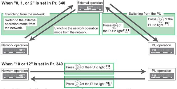
For the switching method from the external terminal, refer to *the inverter manual (applied)*. Refer to *page 66* for a switching method from the network.
