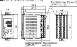
Mount the Product such that the display can be seen properly from the front. To fix the Product to the panel, use the attached mounting bracket.
