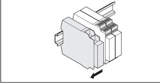
$\Rightarrow$  If there are several modules, slide the modules away from each other individually in the direction of the arrow until the side plug connection is separated.
