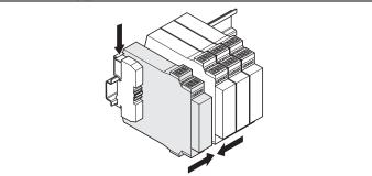
⇒ If there are several modules, slide the modules together individually in the direction of the arrow until the side plug connection latches in.
