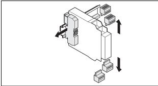
$\Rightarrow$  Remove the removable terminals with wiring and the end clips.
