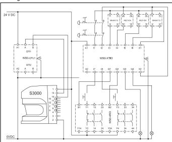
\*: The WS0-4RO cannot be used alone. The WS0-4RO performs the ON/OFF control via the WS0-XTIO. Connect the output terminals (Q1 to Q4) of the WS0-XTIO to the input terminals (B1 and B2).
