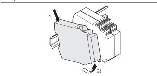
$\Rightarrow$  Press the module downwards at the rear (1)) and remove it from the DIN rail in the direction of the arrow while keeping it pressed down (2)).
