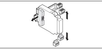
$\Rightarrow$  Remove the removable terminals with wiring and the end clips.
