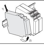
$\Rightarrow$  Press the module downwards at the rear (1)) and remove it from the DIN rail in the direction of the arrow while keeping it pressed down (2)).
