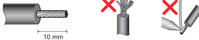
Cable sheath stripping length
