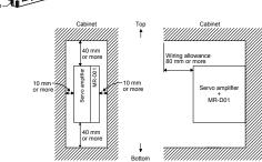
4. Electrical Installation and configuration diagram
